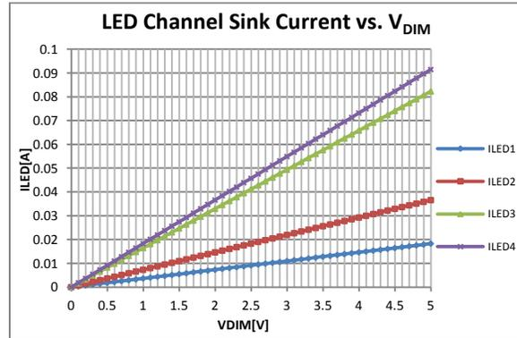
Figure 14. Measured LED Channel Sink Current vs. V<sub>DIM</sub> (R<sub>CS</sub> = 10 Ω)
