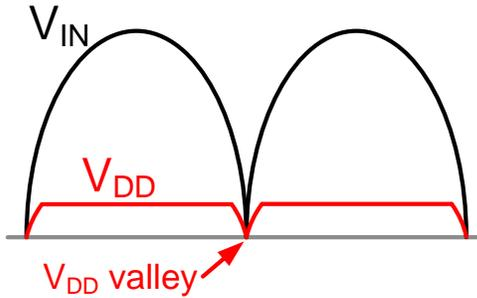
Figure 12. V<sub>DD</sub> Ripple without C<sub>VDD</sub>
