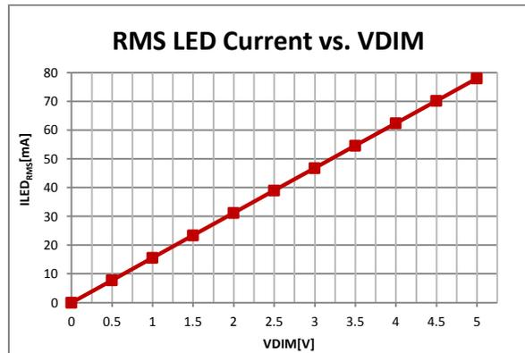
Figure 15. Current vs. V<sub>DIM</sub> (Simulation results: R<sub>CS</sub>=10 Ω / V<sub>AC</sub> = 120 V)
