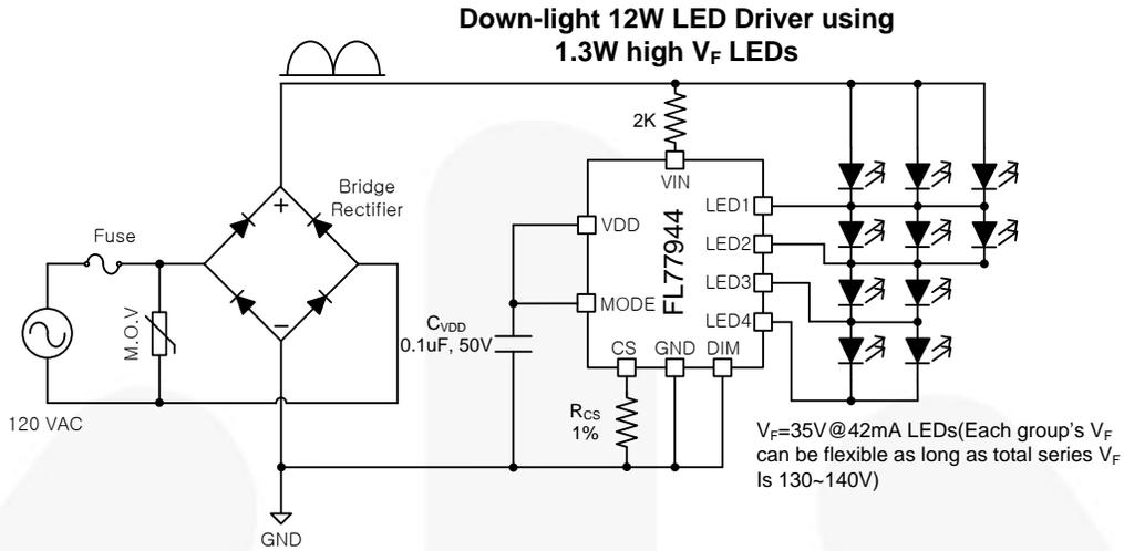
Figure 1. 12 W at 120 V<sub>AC</sub> LED Down-Light Application
