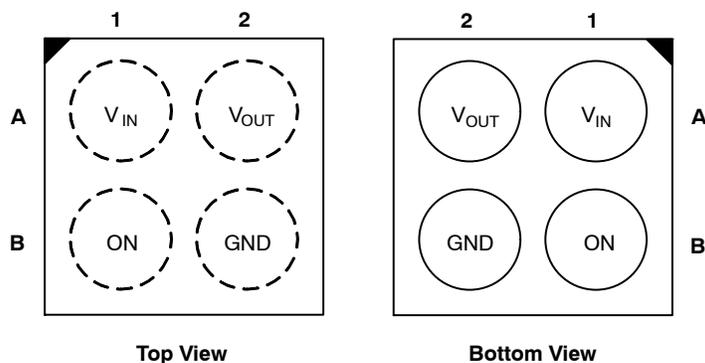
Figure 4. Pin Configuration
