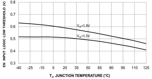
Figure 11. EN Input Logic Low Threshold Vs. Temperature
