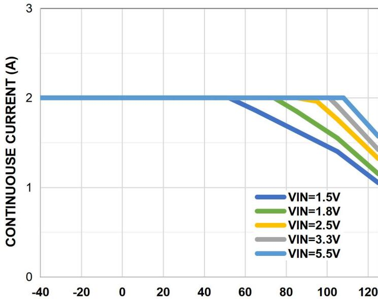
Note. This graph is based on a high effective thermal conductivity four-layer test board per JEDEC 51-7.
