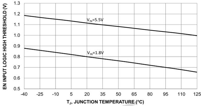
Figure 10. EN Input Logic High Threshold Vs. Temperature
