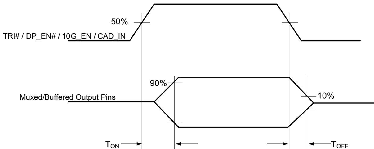
**Figure 1. Control Line Change to Switched Signals**
