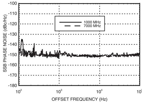
[1] Phase Noise Floor vs Offset Frequency over temperature
