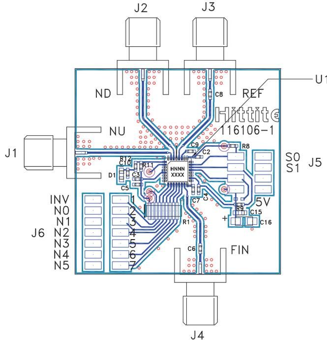
The circuit board used in the final application should use RF circuit design techniques. Signal lines should have 50 ohm impedance while the package backside ground paddle should be connected directly to the ground plane similar to that shown. A sufficient number of via holes should be used to connect the top and bottom ground planes. The evaluation circuit board shown is available from Hittite upon request.
