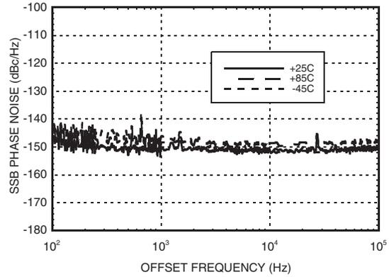
**Phase Noise Floor vs Offset Frequency
