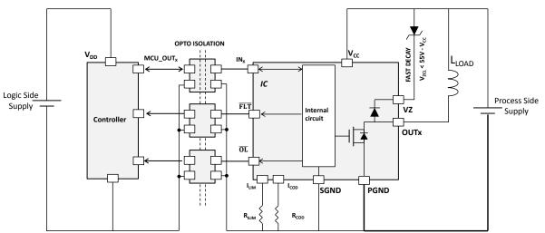
Figure 6. Application circuit (fast decay enabled by TVS between VZ and PGND).
