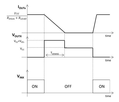
Figure 15. V<sub>OUT</sub> and I<sub>OUT</sub> in case of fast demagnetization (fast decay)
