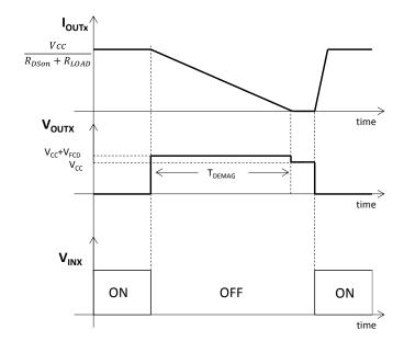
Figure 13. V<sub>OUT</sub> and I<sub>OUT</sub> in case of slow demagnetization
