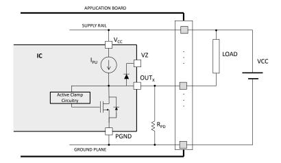
Figure 14. Active clamp equivalent principle schematic.
