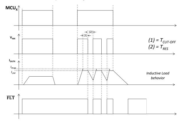
Figure 9. Cut-off signalization behavior on FLT
