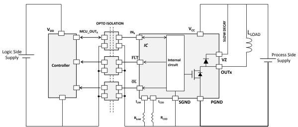
Figure 7. Application circuit (fast decay disabled by Vz shorted to supply rail) .
