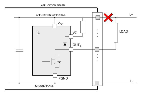
Figure 12. VCC wire break
