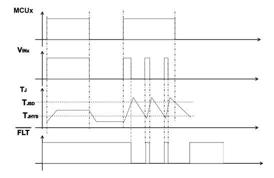
Figure 8. Thermal protection signalization behavior on FLT
