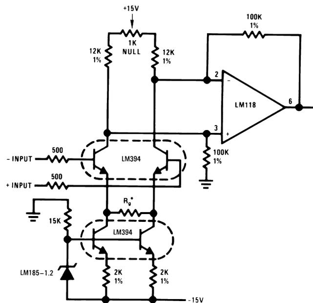
$$*Gain \geq \frac{200K}{R_g} \text{ for } 1.5K \leq R_g \leq 200K$$
