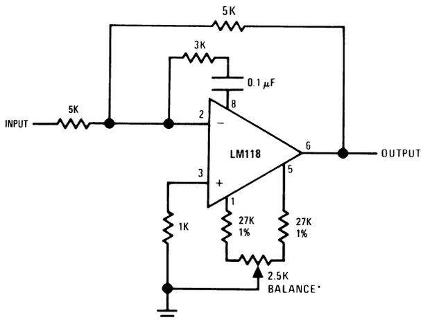
\*Balance circuit necessary for increased slew.
