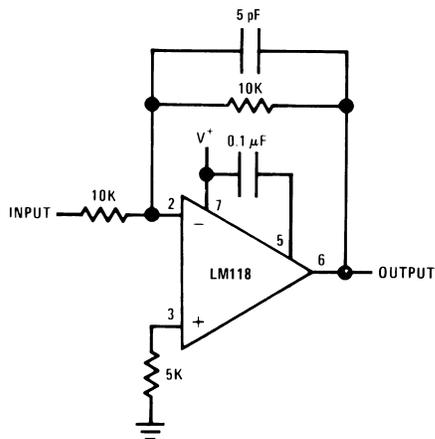
Slew and settling time to 0.1% for a 10V step change is 800 ns.
