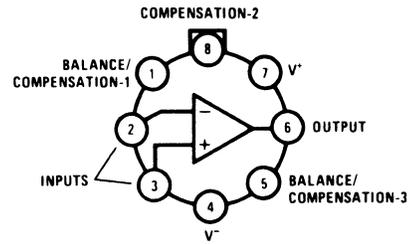
Pin connections shown on schematic diagram and typical applications are for TO-5 package.
