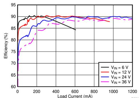
Typical Efficiency, V<sub>OUT</sub> = 12 V
