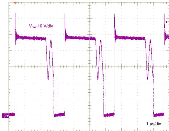
$V_{IN} = 36\text{ V}$   $I_{OUT} = 1\text{ A}$
