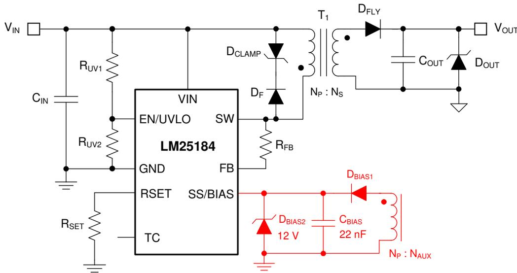
**Figure 7-4. External Bias Supply Using Transformer Auxiliary Winding**
