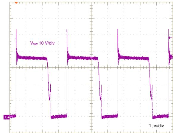
$V_{IN} = 24\text{ V}$   $I_{OUT} = 1\text{ A}$
