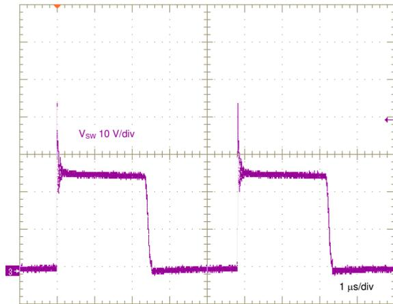
$V_{IN} = 13.5\text{ V}$   $I_{OUT} = 1\text{ A}$
