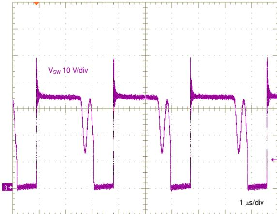
$V_{IN} = 24\text{ V}$        $I_{OUT1} = I_{OUT2} = 0.3\text{ A}$
