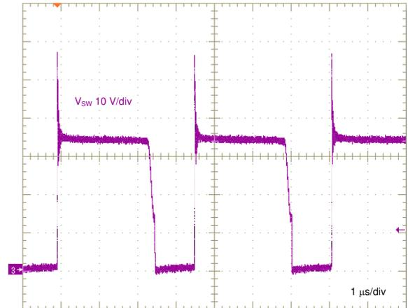
$V_{IN} = 24\text{ V}$        $I_{OUT1} = I_{OUT2} = 0.5\text{ A}$
