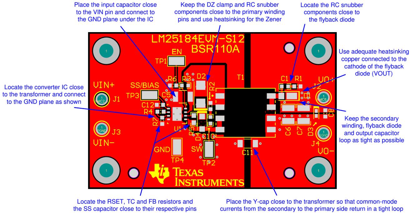
**Figure 10-1. Single-Output PCB Layout Example**
