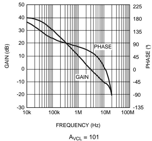
Figure 6. Error Amplifier Gain and Phase
