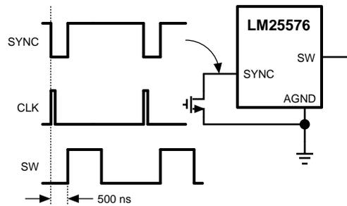
**Figure 9. Sync from External Clock**
