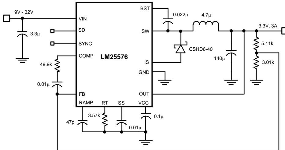
Figure 20. Schematic 3.3 V, 3 A, 1 MHz
