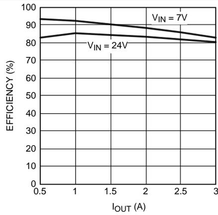
Figure 7. Demoboard Efficiency vs I<sub>OUT</sub> and V<sub>IN</sub>
