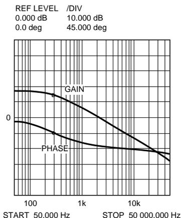
Figure 15. Gain and Phase of Modulator
