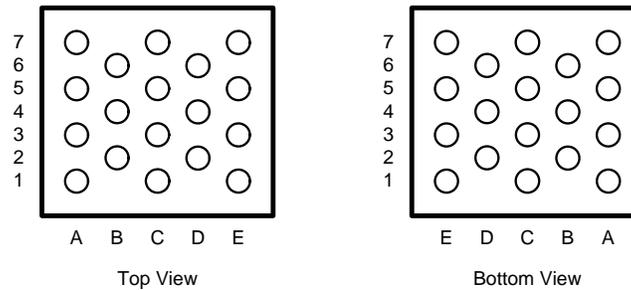
**Figure 3. 18-Bump Thin DSBGA Package**
