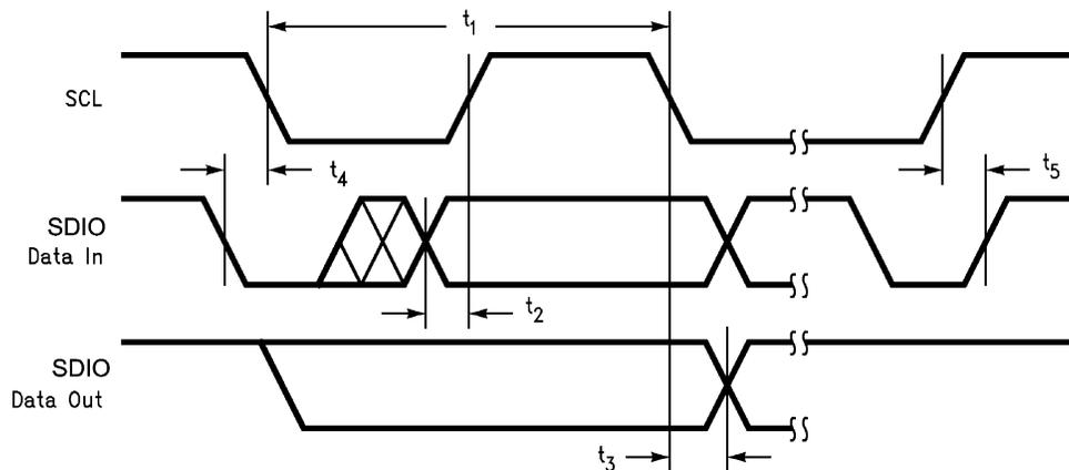
Figure 4. I<sup>2</sup>C Timing Diagram
