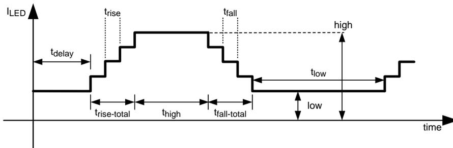
Figure 20. Dimming Waveform
