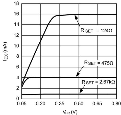
**Figure 24.  $I_{LED}$  vs  $V_{HR}$**
