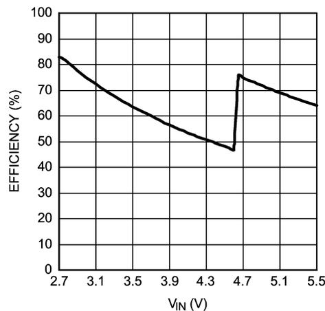
**Figure 27. Efficiency vs  $V_{IN}$**
