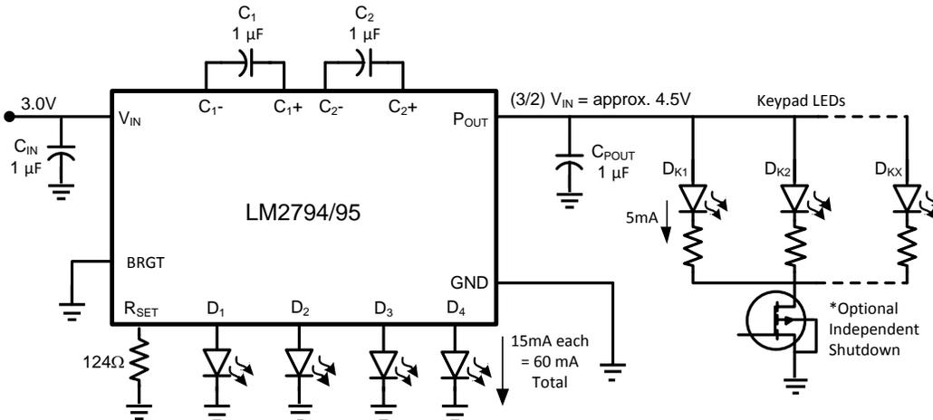
Figure 23. Keypad LEDs Connected to P<sub>OUT</sub>
