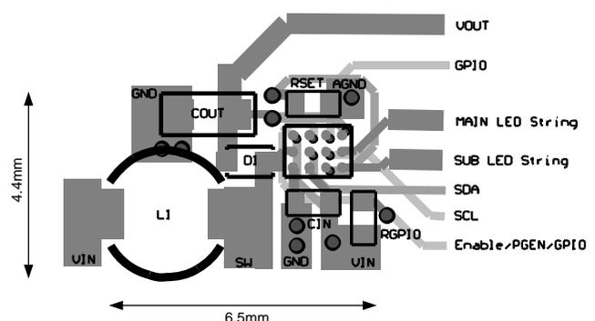
**Figure 2. Typical PCB Layout**
