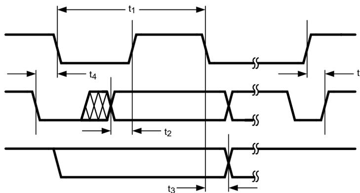
Figure 4. I<sup>2</sup>C Timing
