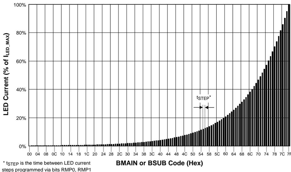
Figure 44. I<sub>MAIN</sub> or I<sub>SUB</sub> vs BMAIN or BSUB Data
