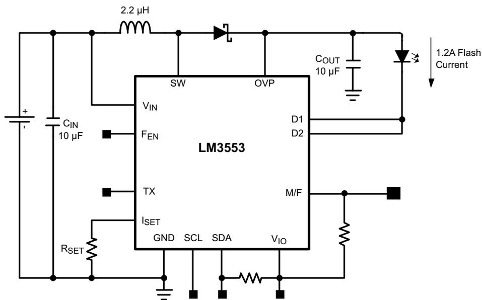
**Figure 24. 1 LED @ 1.2A with Battery Input**
