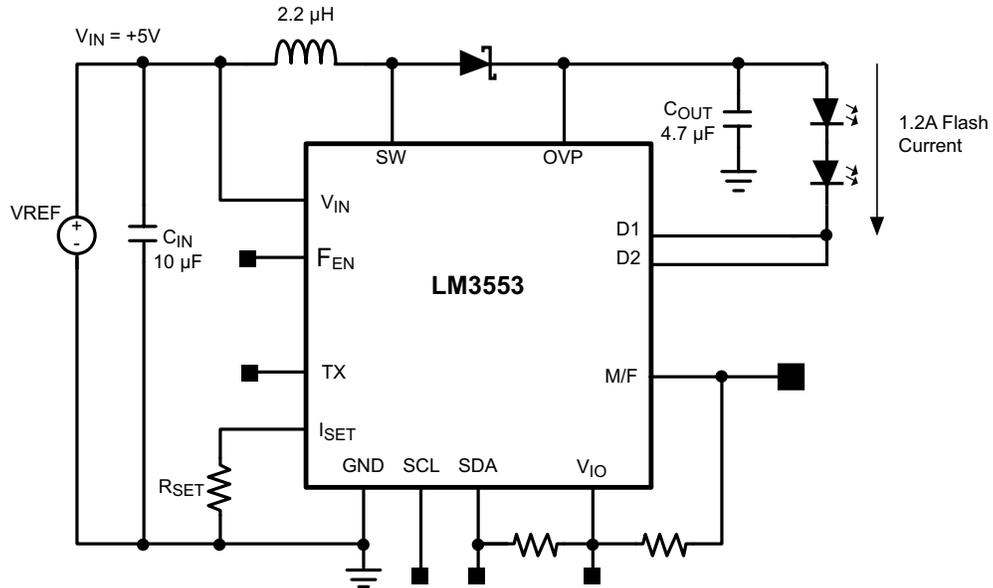
Figure 25. 2 LEDs @ 1.2A with +5V Input
