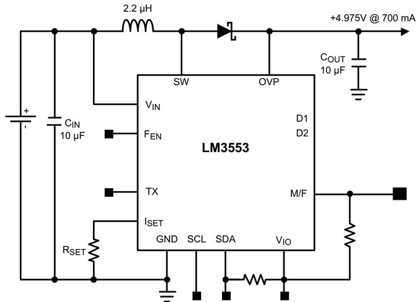
Figure 26. Voltage Mode @ 700mA with Battery Input
