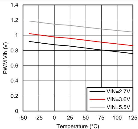
Figure 10. PWM V<sub>IH</sub> vs Temperature
