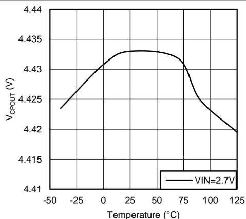
Figure 8. Charge Pump 2X Mode V<sub>CPOUT</sub> vs Temperature
