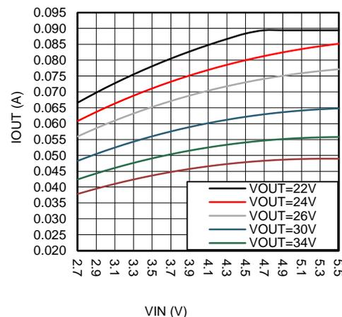
Figure 25. Maximum Output Power (10  $\mu\text{H}$ )
