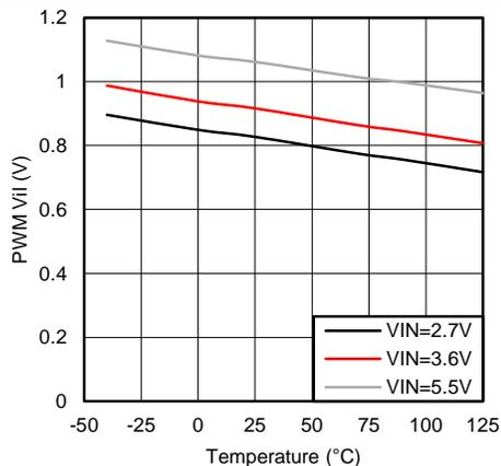
Figure 11. PWM V<sub>IL</sub> vs Temperature
