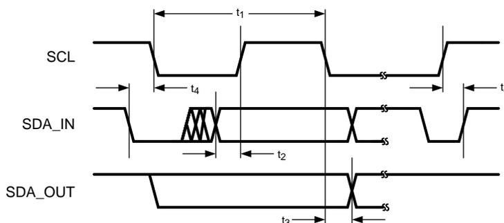
Figure 1. I<sup>2</sup>C-Compatible Interface Timing
