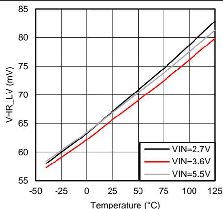
Figure 9. V<sub>HR\_LV</sub> vs Temperature
