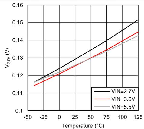
Figure 7. Low Voltage LED  $V_{GTH}$  vs Temperature
