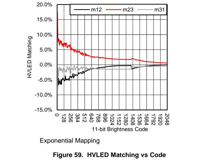
$V_{IN} = 3.6\text{ V}$ ,  $V_{LED} = 3.2\text{ V @ } 20\text{ mA}$ , Typical Application Circuit,  $T_A = 25^\circ\text{C}$ , Full-Scale Current = 20.2 mA unless otherwise specified. Efficiency is  $V_{OUT} \times (I_{HVLED1} + I_{HVLED2} + I_{HVLED3}) / (V_{IN} \times I_{IN})$ , matching curves are  $(\Delta I_{LED\_MAX} / I_{LED\_AVE})$ . See Table 37.
