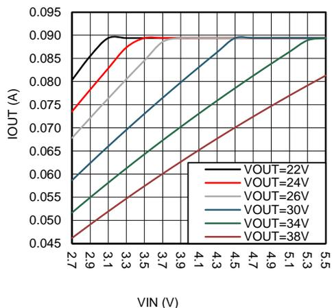
Figure 24. Maximum Output Power (22  $\mu\text{H}$ )
