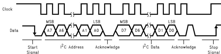
Figure 31. I<sup>2</sup>C Bus Format
