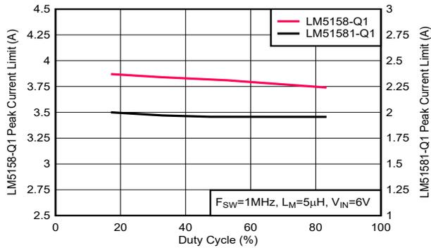
**Figure 8-13. Peak Current Limit vs Duty Cycle**
