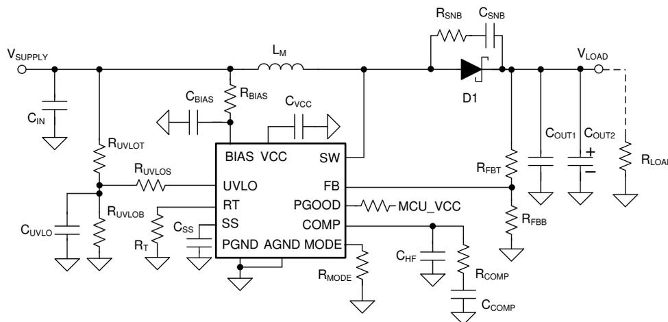
**Figure 10-1. Typical Boost Converter Circuit with Optional Components**
