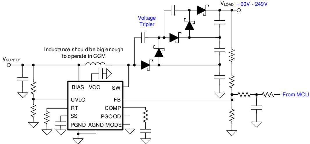
**Figure 10-6. LIDAR Bias Supply 2 (CCM Operation)**
