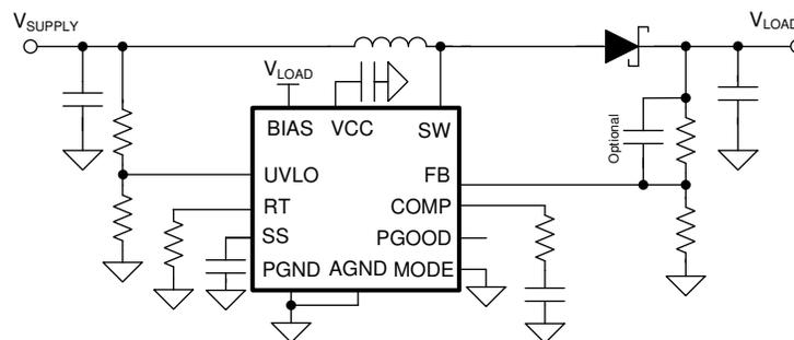
**Figure 9-5. Decrease the Minimum Operating Voltage After Start-Up**
