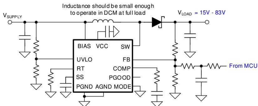
**Figure 10-5. LIDAR Bias Supply 1 (DCM Operation)**
