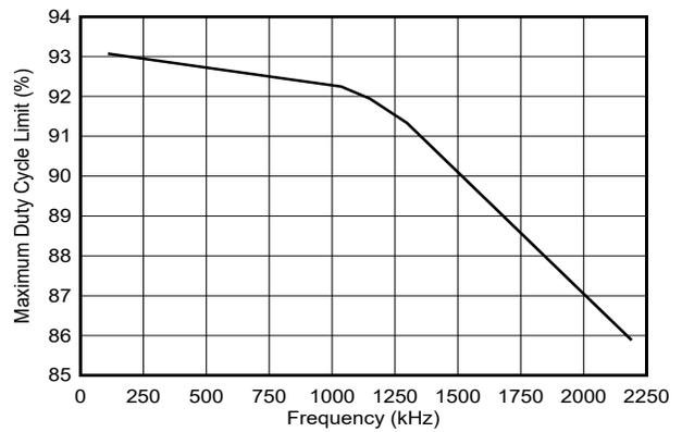
**Figure 8-16. Maximum Duty Cycle Limit vs Frequency**
