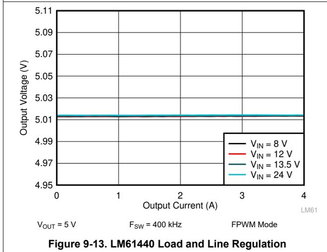
Figure 9-13. LM61440 Load and Line Regulation
