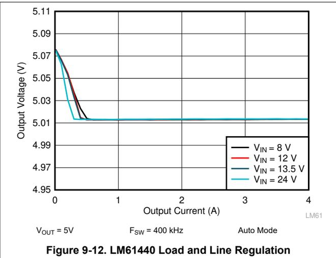
Figure 9-12. LM61440 Load and Line Regulation
