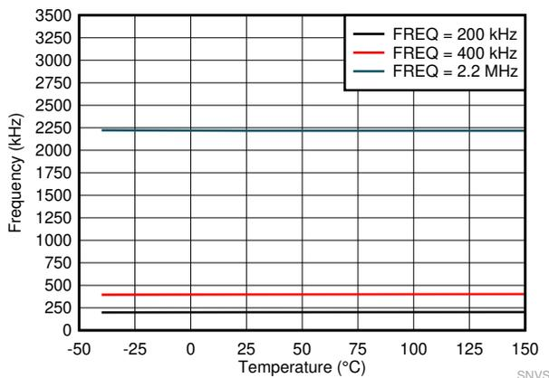
Figure 7-5. Switching Frequency Set by RT Resistor
