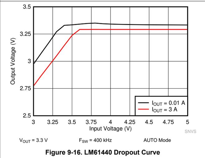
Figure 9-16. LM61440 Dropout Curve
