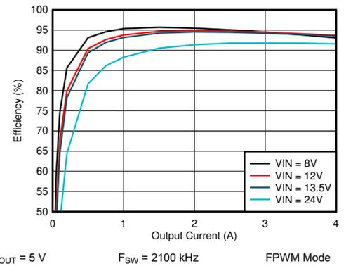
$V_{OUT} = 5\text{ V}$   $F_{SW} = 2100\text{ kHz}$  FPWM Mode
