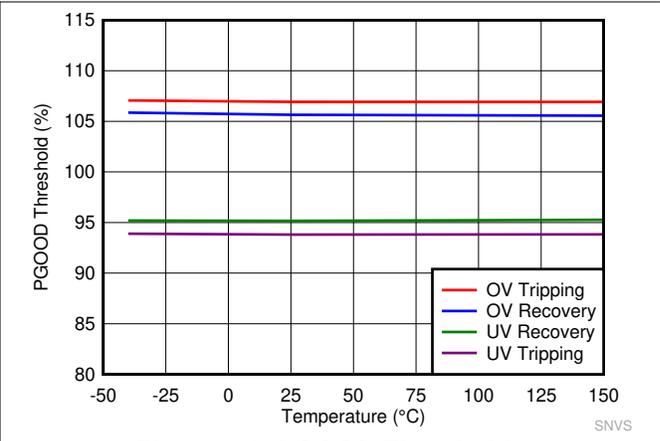
Figure 7-8. PGOOD Thresholds
