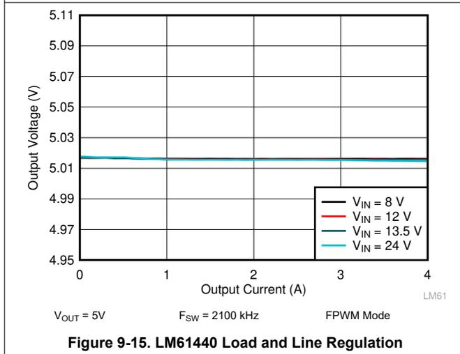
Figure 9-15. LM61440 Load and Line Regulation
