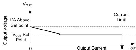
In auto mode, once output current drops below approximately 1/10th the rated current of the part, output resistance increases so that output voltage is 1% high while the buck is completely unloaded.
