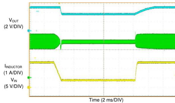
**Figure 8-10. Recovery From Dropout ( $V_{OUT} = 5\text{ V}$ ,  $I_{OUT} = 4\text{ A}$ ,  $V_{IN} = 13.5\text{ V}$  to  $4\text{ V}$  to  $13.5\text{ V}$ )**
