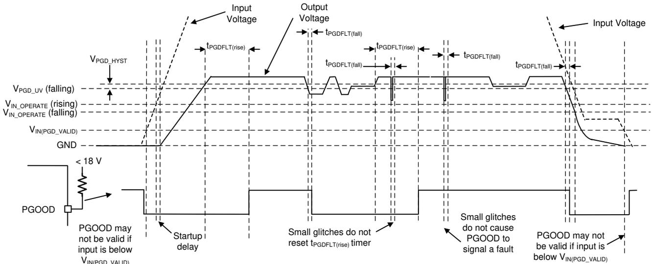
Figure 8-6. PGOOD Timing Diagram (Excludes OV Events)
