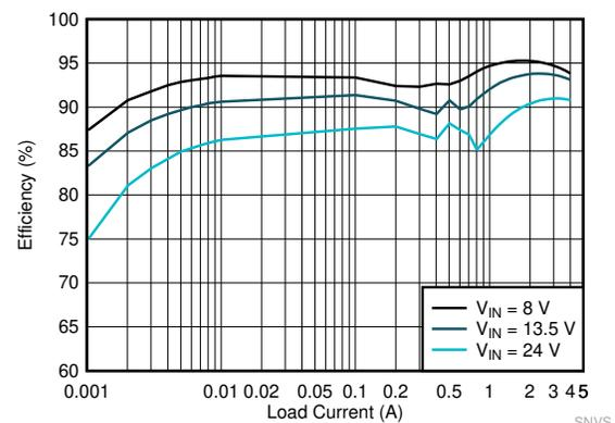
**Efficiency  $V_{OUT} = 5\text{ V}$ ,  $F_{SW} = 2200\text{ kHz}$**
