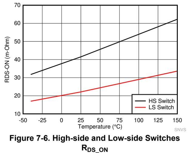
Figure 7-6. High-side and Low-side Switches  $R_{DS\_ON}$
