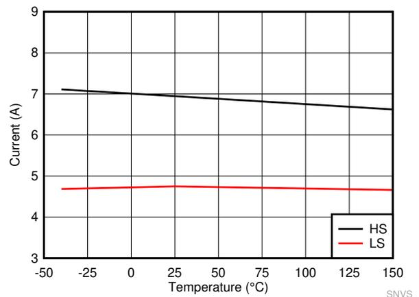
Figure 7-4. LM61440 High-side and Low-side Current Limits
