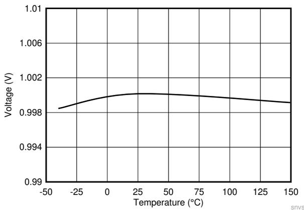
Figure 7-3. Feedback Voltage
