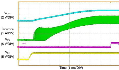
$V_{OUT} = 3.3\text{ V}$        $F_{SW} = 2100\text{ kHz}$       FPWM Mode
