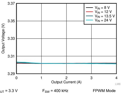
$V_{OUT} = 3.3\text{ V}$   $F_{SW} = 400\text{ kHz}$  FPWM Mode
