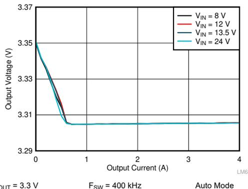
$V_{OUT} = 3.3\text{ V}$   $F_{SW} = 400\text{ kHz}$  Auto Mode
