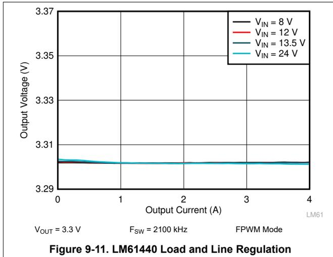
Figure 9-11. LM61440 Load and Line Regulation
