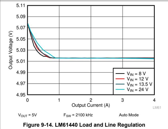
Figure 9-14. LM61440 Load and Line Regulation
