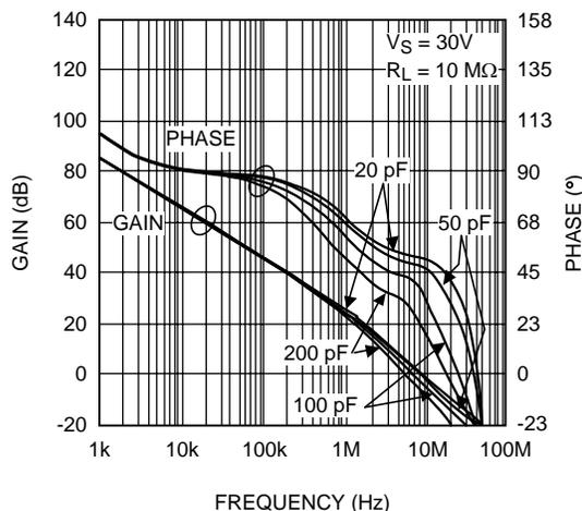
Figure 28. Open-Loop Frequency Response With Various Capacitive Loads
