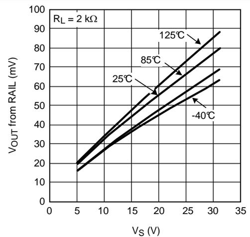
Figure 24. Negative Output Swing vs Supply Voltage
