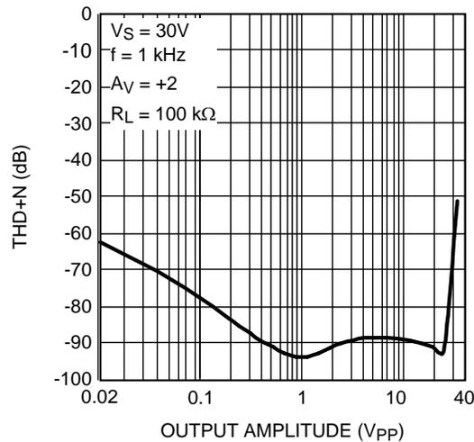
Figure 45. THD+N vs Output Amplitude ( $V_{PP}$ )
