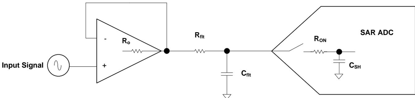
**Figure 50. Drive Amplifier for SAR ADC Schematic**
