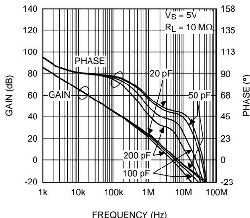
Figure 26. Open-Loop Frequency Response With Various Capacitive Loads
