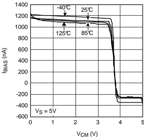
Figure 11.  $I_{BIAS}$  vs  $V_{CM}$
