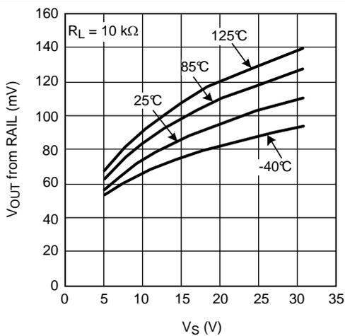
Figure 23. Positive Output Swing vs Supply Voltage
