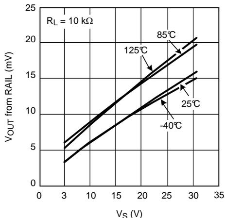
Figure 25. Negative Output Swing vs Supply Voltage
