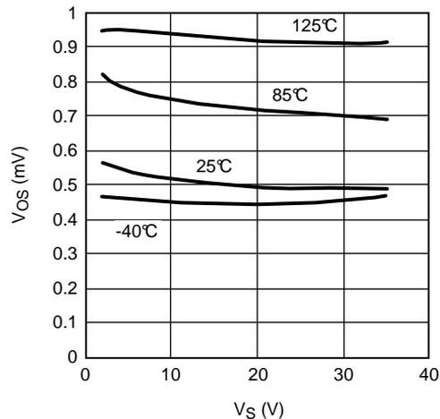
Figure 9.  $V_{OS}$  vs  $V_S$  (Unit 2)
