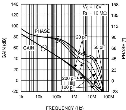
Figure 27. Open-Loop Frequency Response With Various Capacitive Loads
