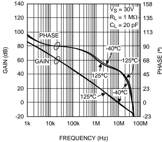
Figure 31. Open-Loop Frequency Response at Various Temperatures
