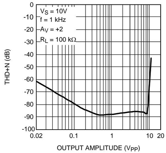
Figure 44. THD+N vs Output Amplitude ( $V_{PP}$ )
