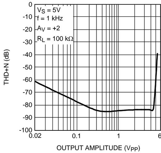
Figure 43. THD+N vs Output Amplitude ( $V_{PP}$ )
