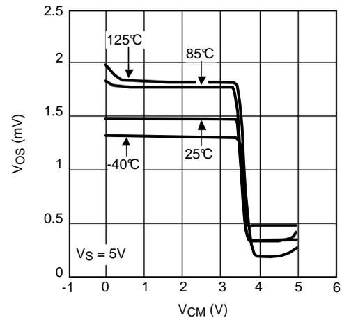
Figure 4.  $V_{OS}$  vs  $V_{CM}$  (Unit 3)
