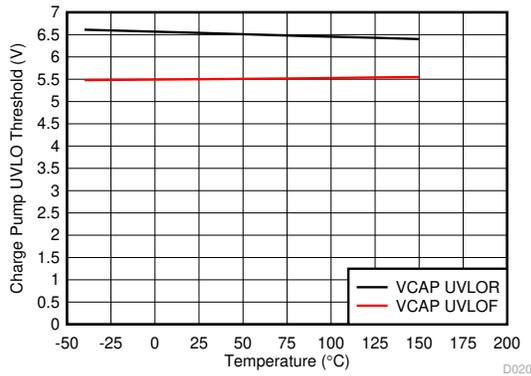
Figure 7-13. Charge Pump UVLO Threshold vs Temperature
