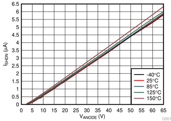
Figure 7-1. Shutdown Supply Current vs Supply Voltage
