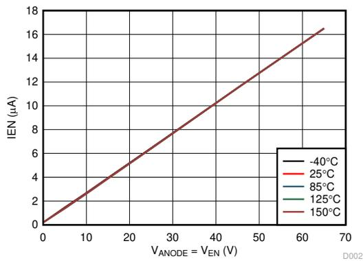
Figure 7-3. Enable Sink Current vs Supply Voltage
