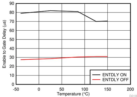
Figure 7-11. Enable to Gate Delay vs Temperature
