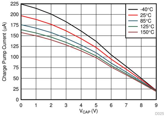
Figure 7-7. Charge Pump V-I Characteristics at ANODE = 3.2 V
