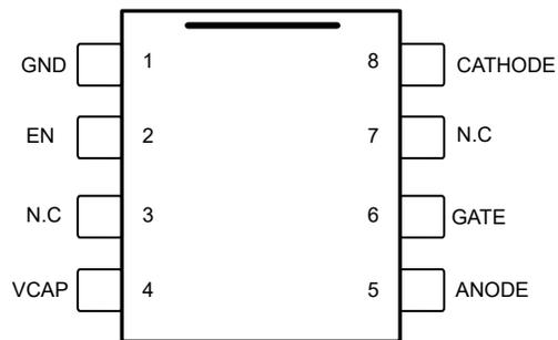
**Figure 5-1. D Package, 8-Pin SOIC Top View**
