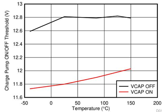
Figure 7-12. Charge Pump ON/OFF Threshold vs Temperature
