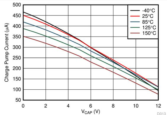
Figure 7-6. Charge Pump V-I Characteristics at ANODE >= 12 V
