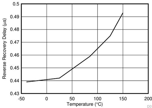
Figure 7-9. Reverse Current Blocking Delay vs Temperature
