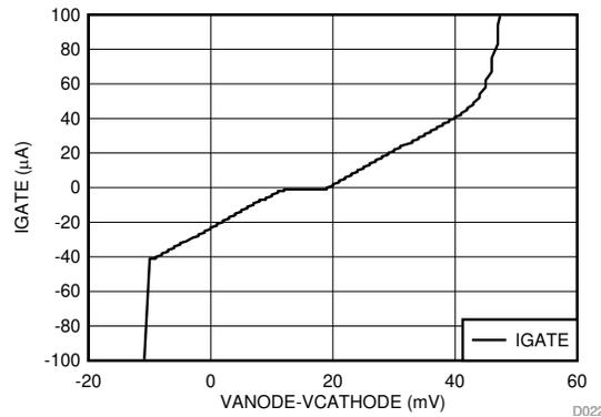
Figure 7-15. Gate Current vs Forward Voltage Drop
