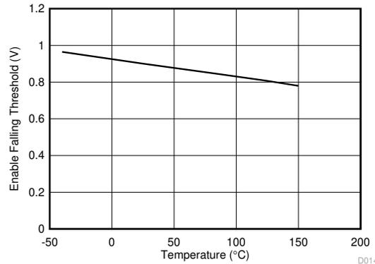
Figure 7-8. Enable Falling Threshold vs Temperature
