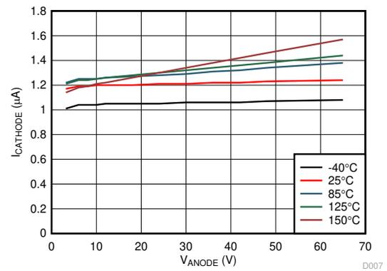
Figure 7-4. CATHODE Sink Current vs Supply Voltage
