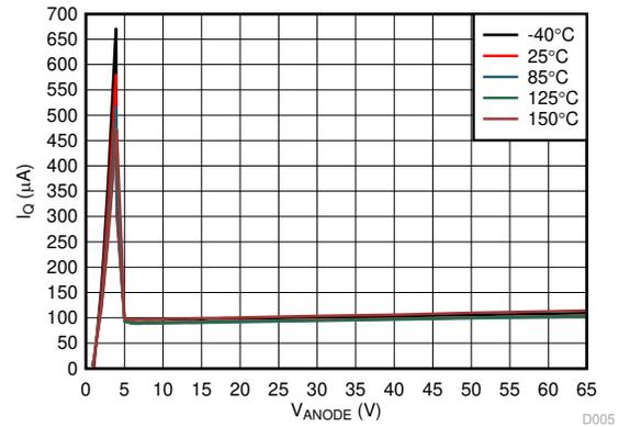
Figure 7-2. Operating Quiescent Current vs Supply Voltage
