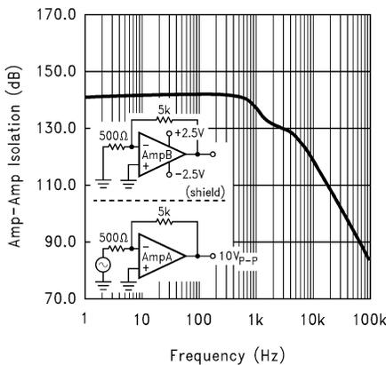
**Figure 5-11. Amp to Amp Isolation vs Frequency**
