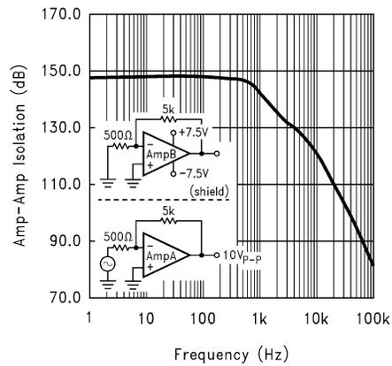
**Figure 5-10. Amp to Amp Isolation vs Frequency**
