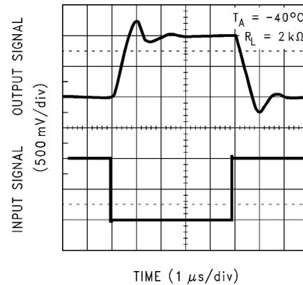
**Figure 5-32. Inverting Large Signal Response**
