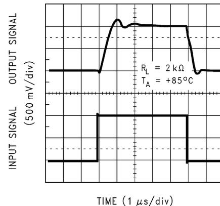
**Figure 5-24. Non-Inverting Large Signal Response**
