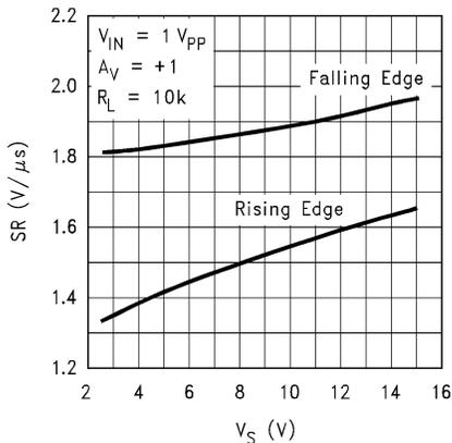
**Figure 5-23. Slew Rate vs Supply Voltage**
