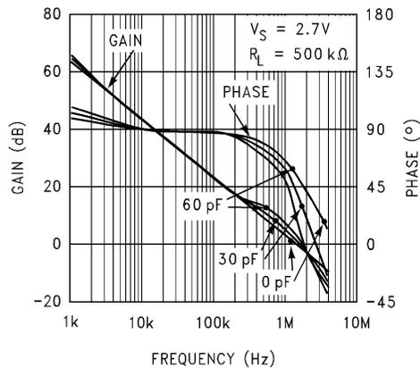
**Figure 5-21. Gain and Phase vs Capacitive Load**
