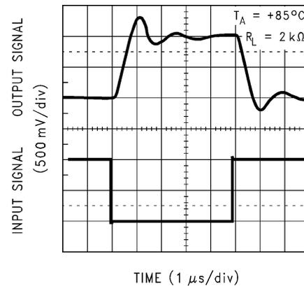
**Figure 5-30. Inverting Large Signal Response**
