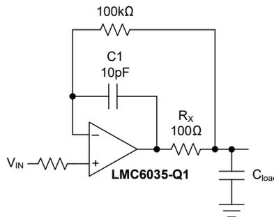
**Figure 7-1.  $R_x$ ,  $C_x$  Improve Capacitive Load Tolerance**
