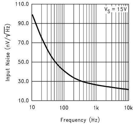
**Figure 5-8. Input Noise vs Frequency**
