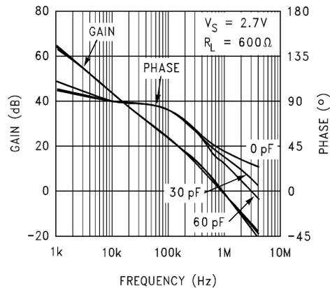
**Figure 5-22. Gain and Phase vs Capacitive Load**
