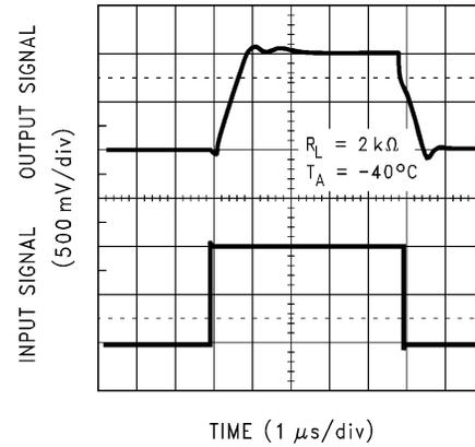
**Figure 5-26. Non-Inverting Large Signal Response**
