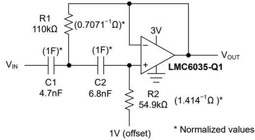
Figure 7-8. 2-Pole, 300Hz, Sallen and Key, High-Pass Filter
