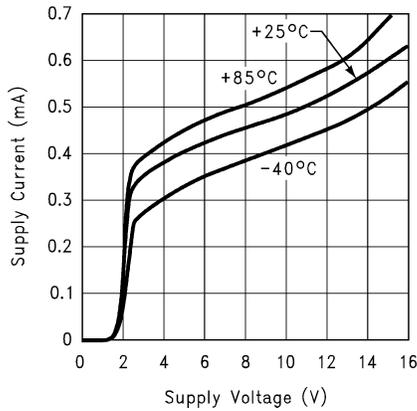
**Figure 5-1. Supply Current vs Supply Voltage (Per Amplifier)**
