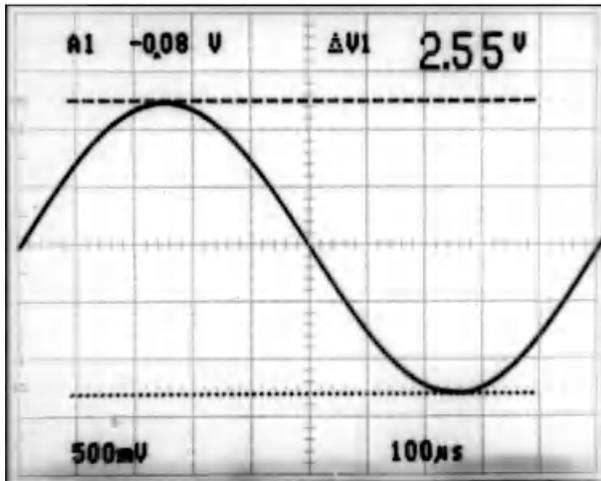
Figure 7-4. Output Swing Performance of the LMC6035-Q1 per the Circuit of Figure 7-3
