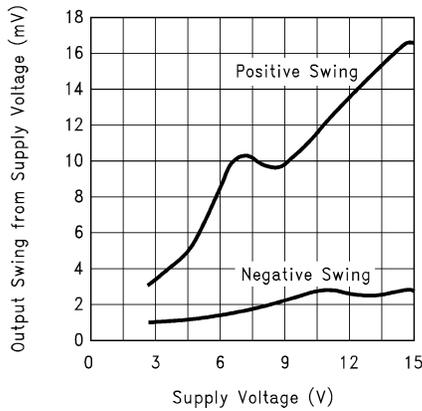
**Figure 5-7. Output Voltage Swing vs Supply Voltage**
