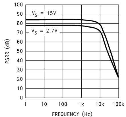
**Figure 5-12. +PSRR vs Frequency**
