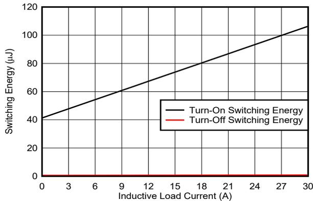
Figure 5-11. Half-Bridge Switching Energy vs Inductive Load Current
