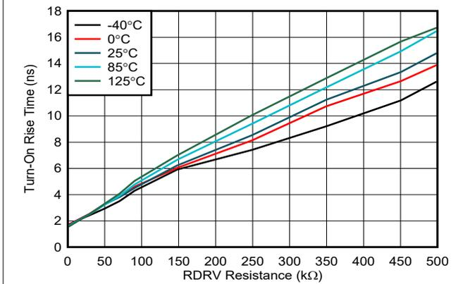
**Figure 5-3. Turn-On Rise Time vs Drive-Strength Resistance**
