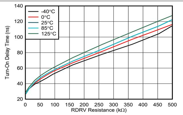
**Figure 5-2. Turn-On Delay Time vs Drive-Strength Resistance**
