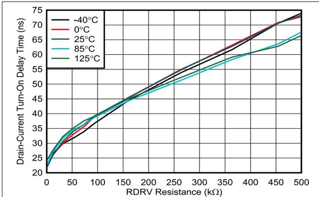
**Figure 5-1. Drain-Current Turn-On Delay Time vs Drive-Strength Resistance**
