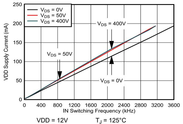
Figure 5-10. VDD Supply Current vs IN Switching Frequency
