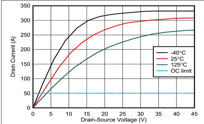
**Figure 5-5. Drain Current vs Drain-Source Voltage**
