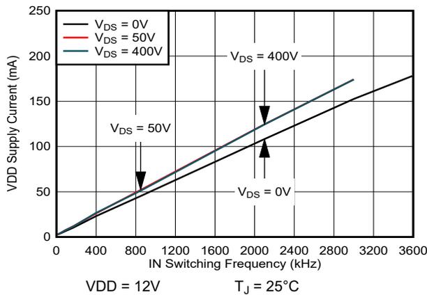
Figure 5-9. VDD Supply Current vs IN Switching Frequency
