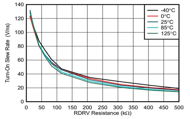
**Figure 5-4. Turn-On Slew Rate vs Drive-Strength Resistance**
