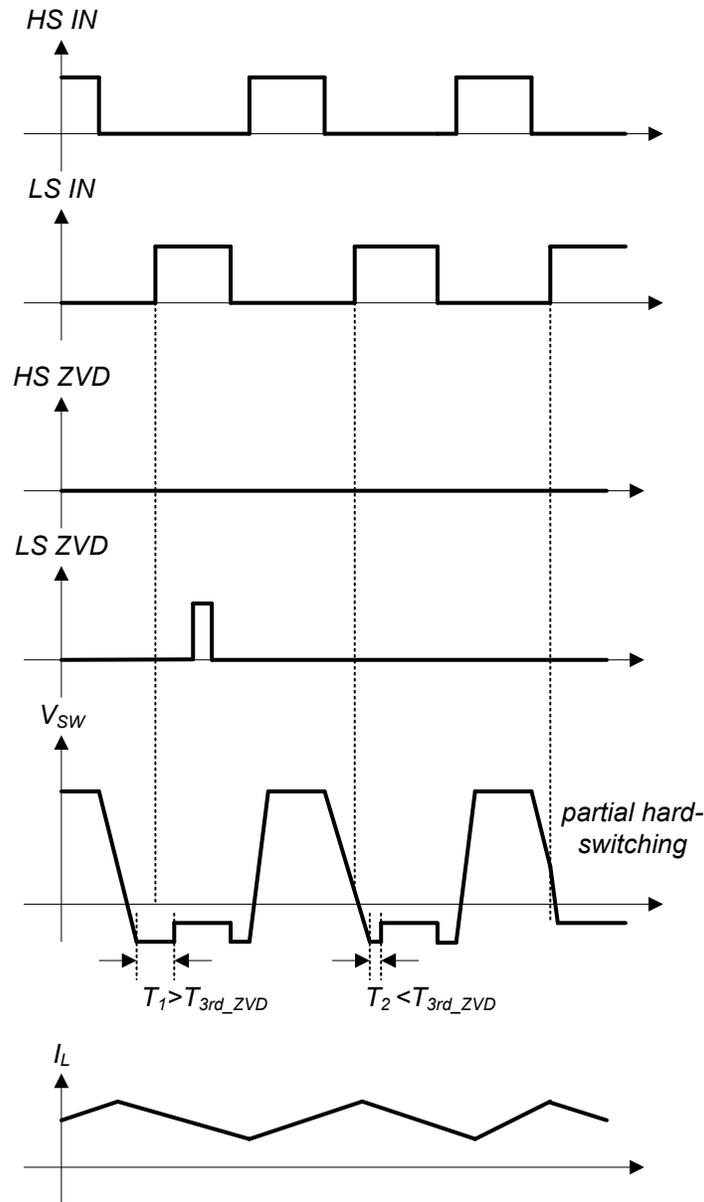
**Figure 7-8. ZVD Function in a CCM Buck Converter**
