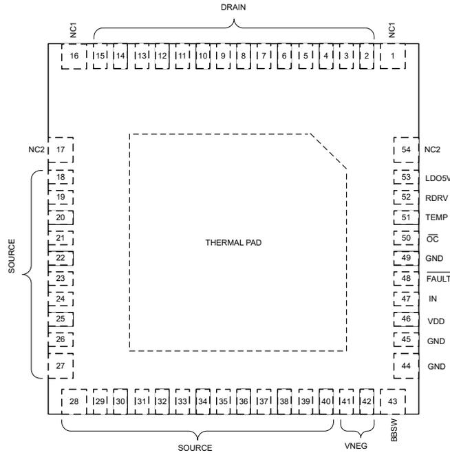
**Figure 4-1. LMG3422R050 RQZ Package, 54-Pin VQFN (Top View)**
