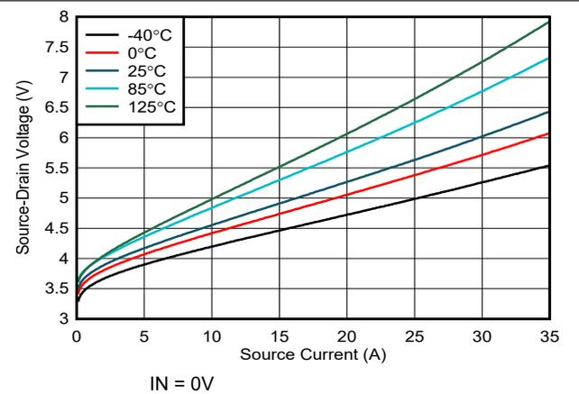
**Figure 5-6. Off-State Source-Drain Voltage vs Source Current**
