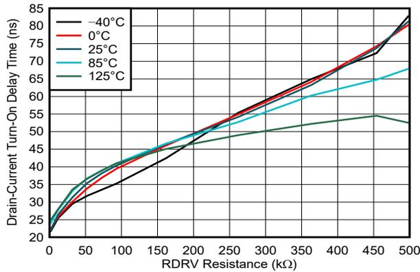
**Figure 5-1. Drain-Current Turn-On Delay Time vs Drive-Strength Resistance**
