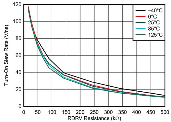
**Figure 5-4. Turn-On Slew Rate vs Drive-Strength Resistance**
