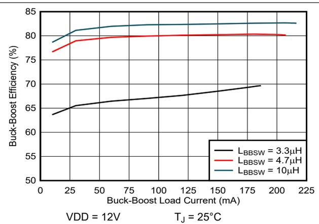
Figure 8-4. Buck-Boost Efficiency vs Load When  $I_{BBSW,PK} = I_{BBSW,PK(high)}$
