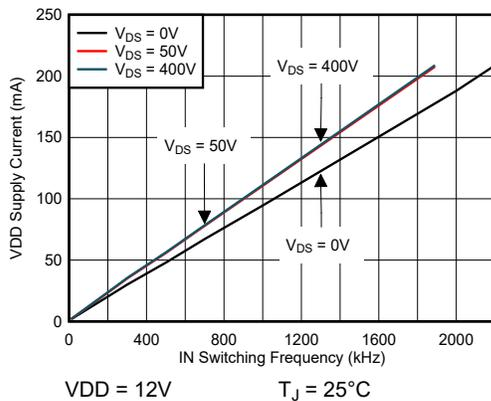
Figure 5-9. VDD Supply Current vs IN Switching Frequency
