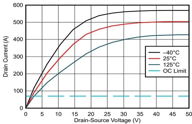
**Figure 5-5. Drain Current vs Drain-Source Voltage**
