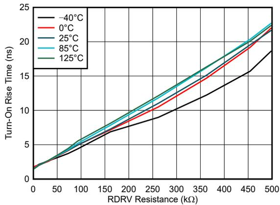
**Figure 5-3. Turn-On Rise Time vs Drive-Strength Resistance**
