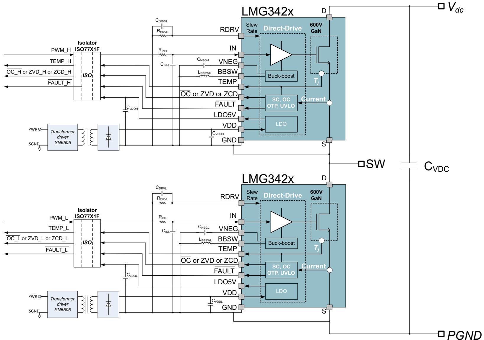
Figure 8-1. Typical Half-Bridge Application With Isolated Power Supply
