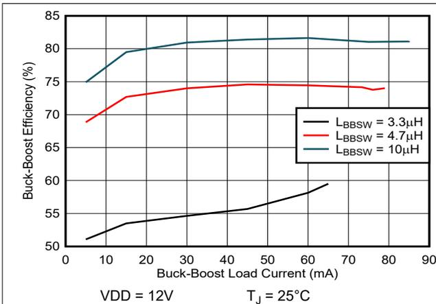
Figure 8-3. Buck-Boost Efficiency vs Load When  $I_{BBSW,PK} = I_{BBSW,PK(low)}$
