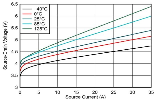
**Figure 5-6. Off-State Source-Drain Voltage vs Source Current**
