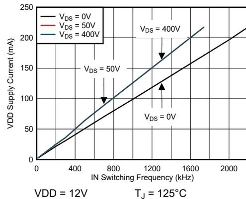
Figure 5-10. VDD Supply Current vs IN Switching Frequency
