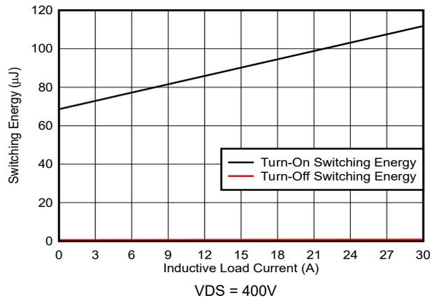
Figure 5-11. Half-Bridge Switching Energy vs Inductive Load Current
