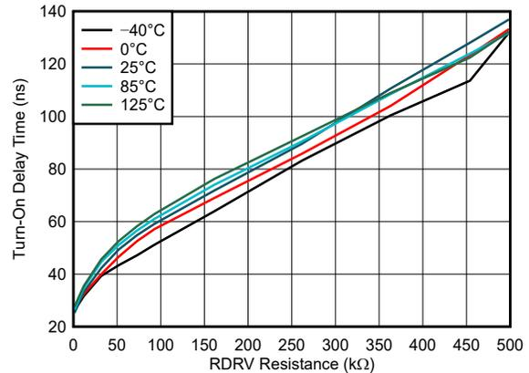
**Figure 5-2. Turn-On Delay Time vs Drive-Strength Resistance**
