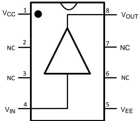
**Figure 2. 8-Pin SOIC (Top View)**
