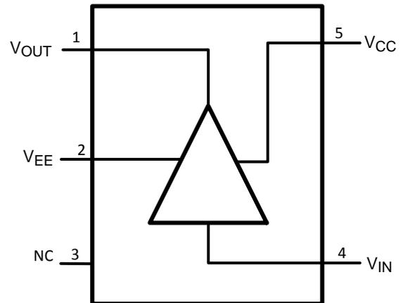
**Figure 3. 5-Pin SOT-23 (Top View)**
