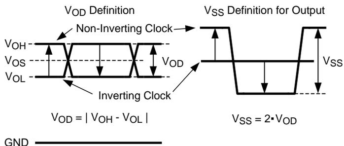
Figure 8. Two Different Definitions for Differential Output Signals
