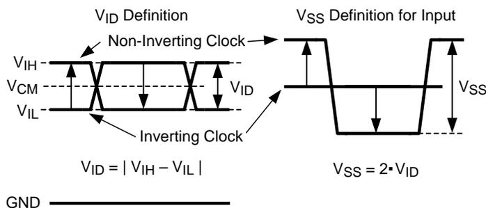
Figure 7. Two Different Definitions for Differential Input Signals
