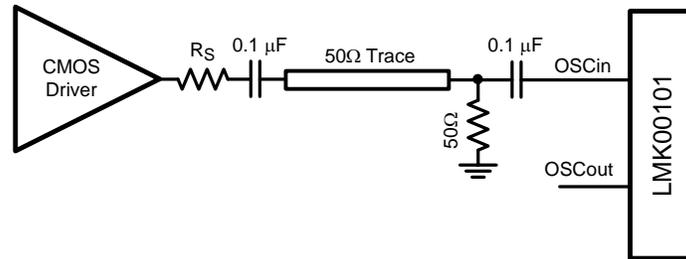
Figure 11. Driving OSCin with a Single-Ended External Clock
