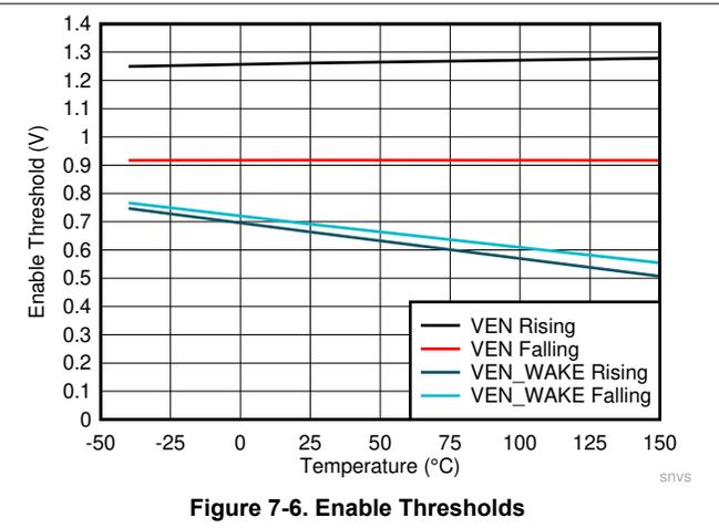
Figure 7-6. Enable Thresholds
