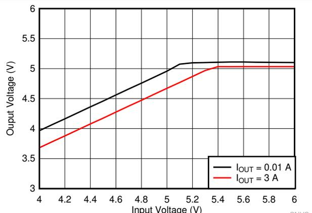
$V_{OUT} = 5V$   $F_{SW} = 2100\text{ kHz}$  AUTO Mode
