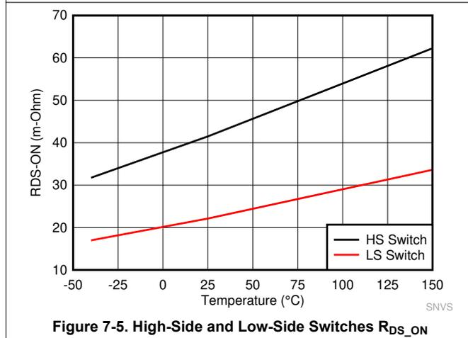
Figure 7-5. High-Side and Low-Side Switches  $R_{DS\_ON}$
