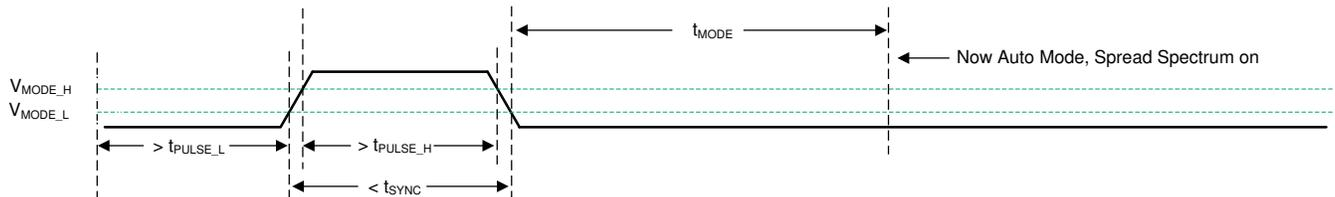
**Figure 8-10. Transition from SYNC Mode to Auto Mode**
