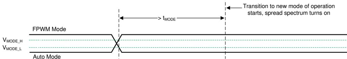
**Figure 8-5. Transition from Auto Mode and FPWM Mode**
