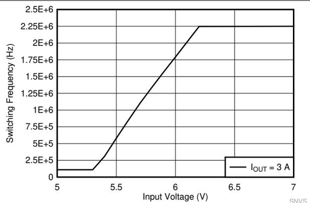
$V_{OUT} = 5V$   $F_{SW} = 2100\text{ kHz}$  AUTO Mode
