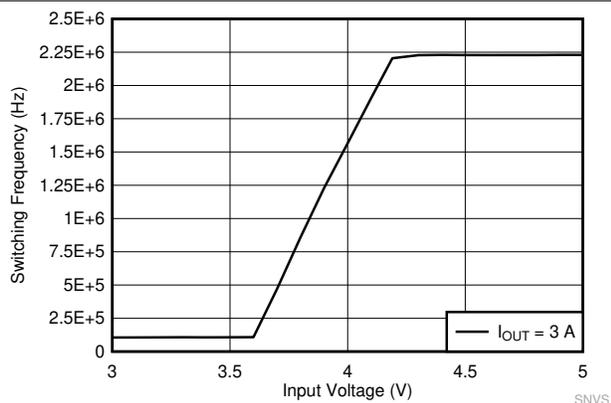
$V_{OUT} = 3.3V$   $F_{SW} = 2100\text{ kHz}$  AUTO Mode
