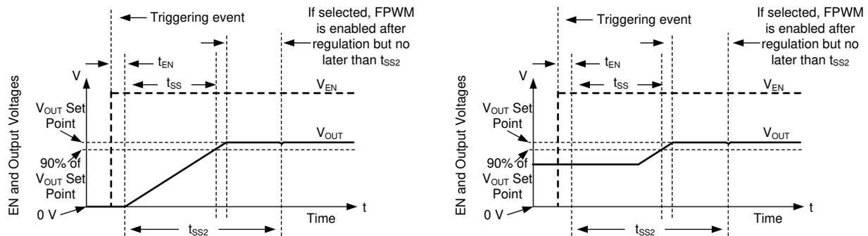
Soft start works with both output voltage starting from 0 V on the left curves, or if there is already voltage on the output, as shown on right. In either case, output voltage must reach within 10% of the desired value  $t_{SS}$  after soft start is initiated. During soft start, FPWM and hiccup are disabled. Both hiccup and FPWM are enabled once output reaches regulation or  $t_{SS2}$ , whichever happens first.
