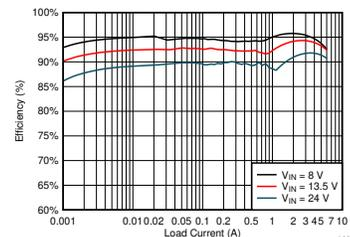
Efficiency:  $V_{\text{OUT}} = 5\text{ V}$ ,  $F_{\text{SW}} = 2.1\text{ MHz}$
