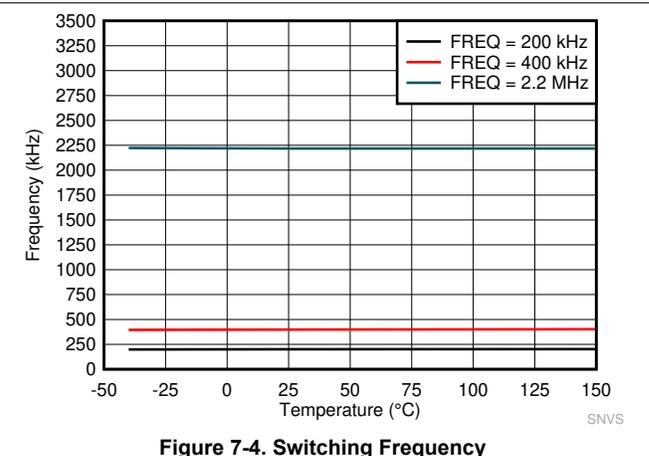
Figure 7-4. Switching Frequency
