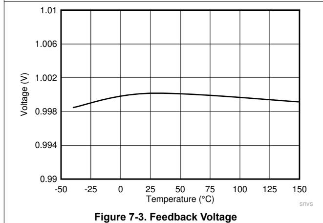
Figure 7-3. Feedback Voltage
