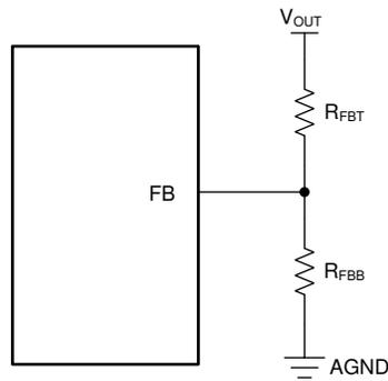
**Figure 8-18. Setting Output Voltage of Adjustable Versions**
