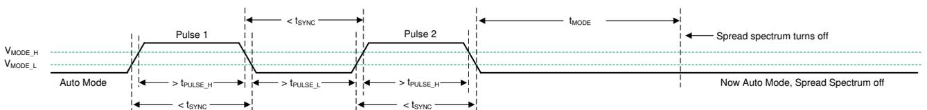
**Figure 8-7. Spread Spectrum Disabled in Auto Mode**
