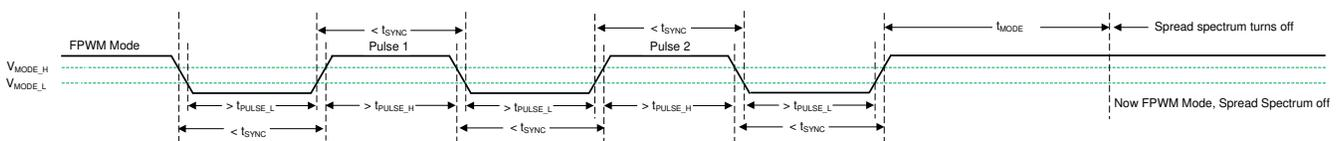
**Figure 8-6. Spread Spectrum Disabled in FPWM Mode**
