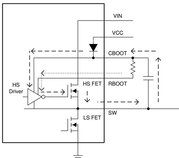
**Figure 8-14. Simplified Circuit Showing How RBOOT Functions**
