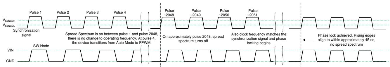
**Figure 8-12. Synchronization Process**
