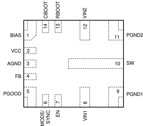
**Figure 6-1. RJR Package 14-Pin VQFN-HR Top View**
