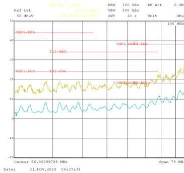
$F_{SW} = 2100 \text{ kHz}$        $V_{OUT} = 5 \text{ V}$        $I_{OUT} = 5 \text{ A}$
