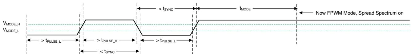
**Figure 8-11. Transition from SYNC Mode to FPWM Mode**
