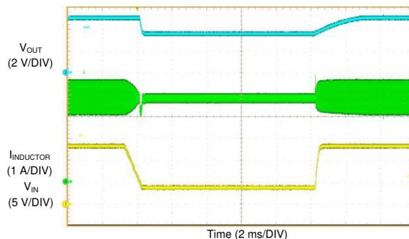
**Figure 8-17. Recovery From Dropout ( $V_{OUT} = 5\text{ V}$ ,  $I_{OUT} = 4\text{ A}$ ,  $V_{IN} = 13.5\text{ V}$  to  $4\text{ V}$  to  $13.5\text{ V}$ )**
