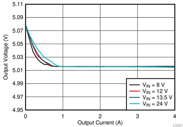
$V_{OUT} = 5V$   $F_{SW} = 2100\text{ kHz}$  Auto Mode
