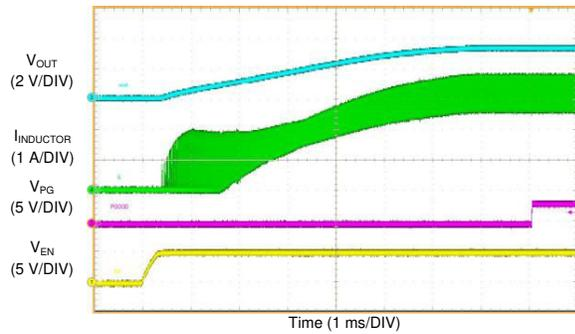
$V_{OUT} = 3.3\text{ V}$        $F_{SW} = 2100\text{ kHz}$       FPWM Mode
