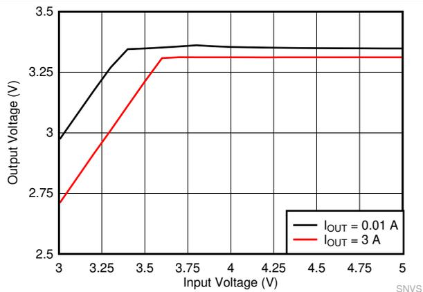
$V_{OUT} = 3.3V$   $F_{SW} = 2100\text{ kHz}$  AUTO Mode
