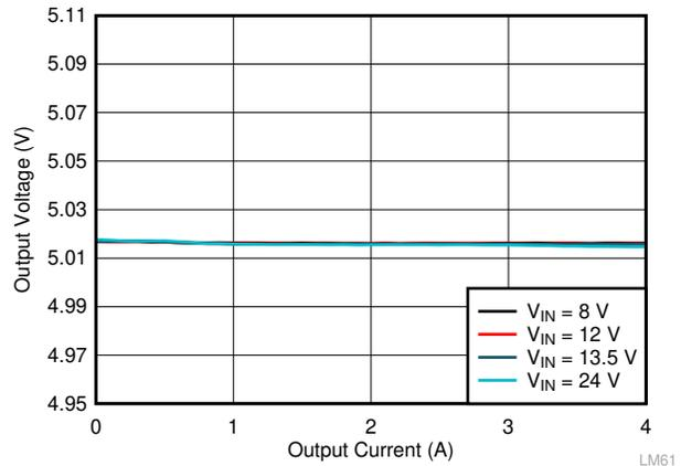
$V_{OUT} = 5V$   $F_{SW} = 2100\text{ kHz}$  FPWM Mode
