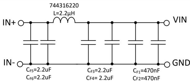
**Figure 9-33. Recommended Input EMI Filter**
