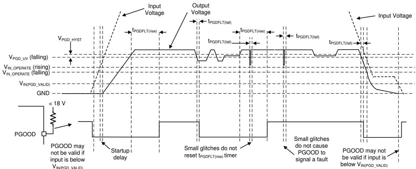
Figure 8-13. PGOOD Timing Diagram (Excludes OV Events)
