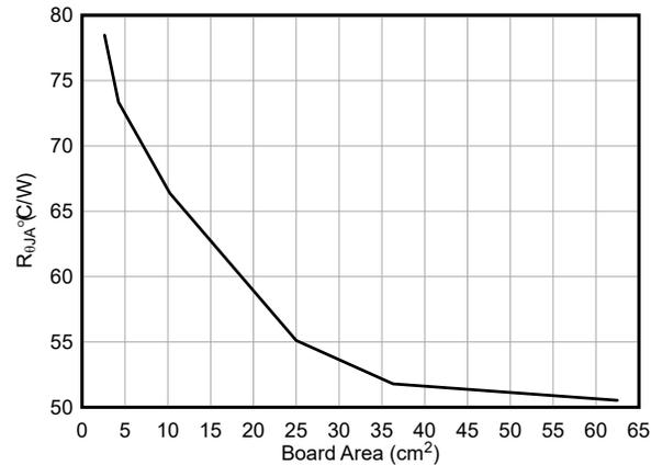
The device operating conditions are as follows: 12-V<sub>IN</sub>, 3.3-V<sub>OUT</sub>, 3-A load, 2.2-MHz, 23°C ambient. 4 layer board, GND plane on Mid-Layer One, 2.8-mil thick copper on each layer, see [LMQ66430-Q1 Buck Controller Evaluation Module User's Guide](#) for copper pattern and thermal vias.
