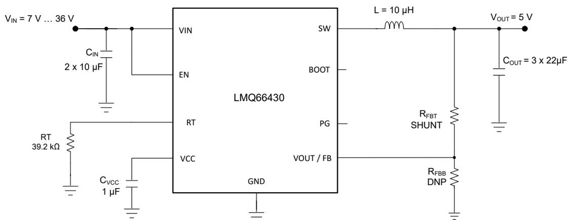
**Figure 9-1. Application Circuit - 5 V (Fixed), 3 A, 400 kHz**
