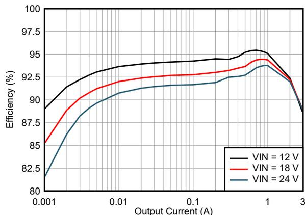
Efficiency:  $V_{OUT} = 5\text{ V}$  (Fixed), 400 kHz
