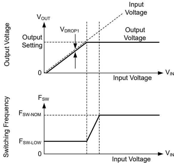
Output voltage and frequency versus input voltage: If there is little difference between input voltage and output voltage setting, the IC reduces frequency to maintain regulation. If input voltage is too low to provide the desired output voltage at  $F_{SW-LOW}$  which is approximately 110-kHz, input voltage tracks output voltage.
