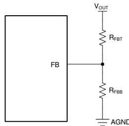
**Figure 8-6. Setting Output Voltage for Adjustable Output Variant**
