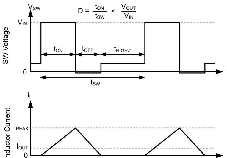
In auto mode, the low-side device is turned off after SW node current is near zero. As a result, after output current is less than half of what inductor ripple can be in CCM, the part operates in DCM, which is equivalent to the statement that diode emulation is active.
