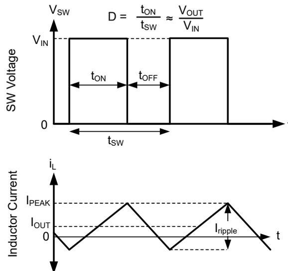
In FPWM mode, continuous conduction (CCM) is possible even if  $I_{OUT}$  is less than half of  $I_{ripple}$ .
