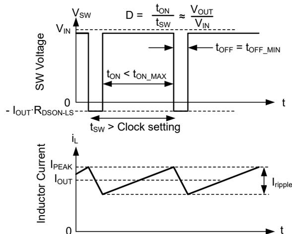
Switching waveforms while in dropout. Inductor current takes longer than a normal clock to reach the desired peak value. As a result, frequency drops. This frequency drop is limited by  $t_{ON-MAX}$ .
