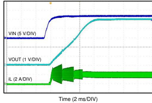
$V_{IN} = 12\text{ V}$        $V_{OUT} = 5\text{ V}$        $I_{OUT} = 2\text{ A}$
