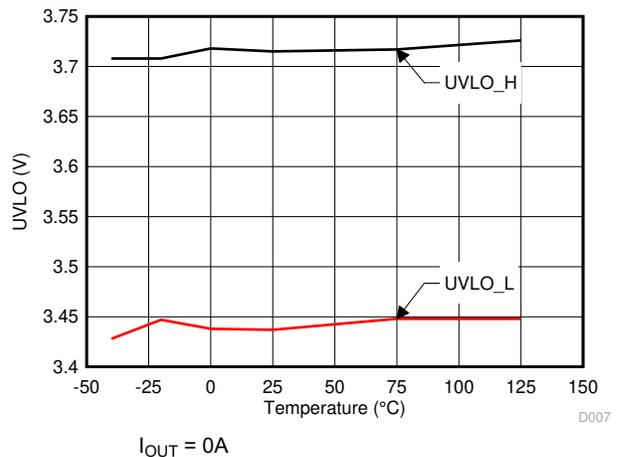
Figure 5-12. UVLO Threshold
