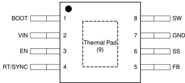
Figure 4-1. DDA Package 8-Pin (HSOIC) Top View
