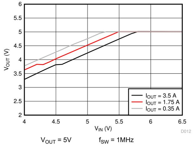
Figure 5-8. Dropout Curve
