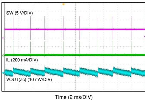
$V_{IN} = 12\text{ V}$        $V_{OUT} = 5\text{ V}$        $I_{OUT} = 0\text{ A}$
