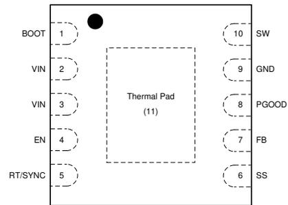
Figure 4-2. DPR Package 10-Pin (WSO) Top View
