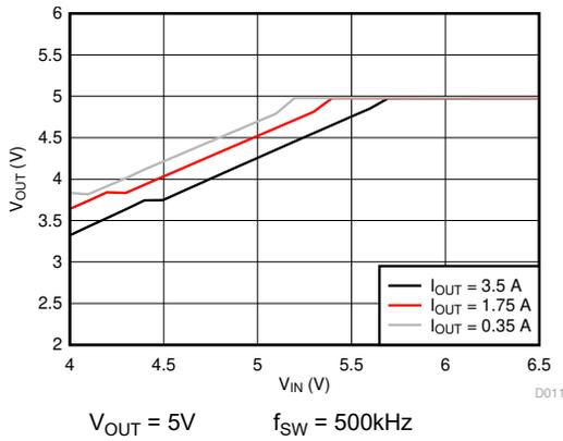
Figure 5-7. Dropout Curve
