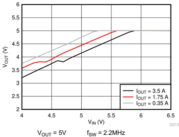
Figure 5-9. Dropout Curve
