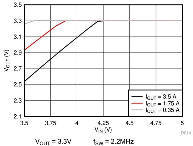
Figure 5-10. Dropout Curve
