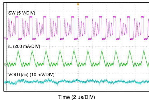
$V_{IN} = 12\text{ V}$        $V_{OUT} = 5\text{ V}$        $I_{OUT} = 100\text{ mA}$
