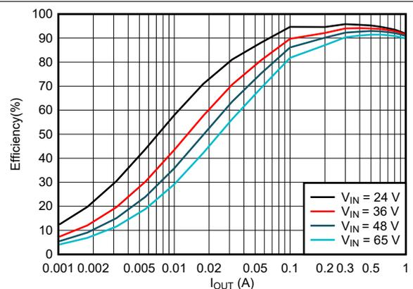
$f_{SW} = 400\text{ kHz}$      $V_{OUT} = 12\text{ V}$     LMR51610XF
