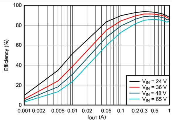
$f_{SW} = 1.1\text{ MHz}$      $V_{OUT} = 12\text{ V}$     LMR51610YF
