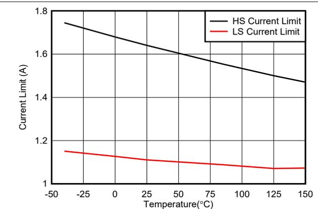
Figure 6-18. HS and LS Current Limit Versus Temperature
