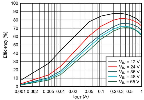
$f_{SW} = 1.1\text{ MHz}$      $V_{OUT} = 3.3\text{ V}$     LMR51610YF
