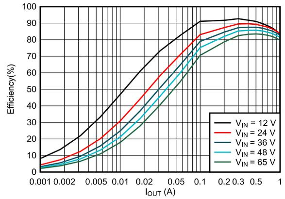
$f_{SW} = 400\text{ kHz}$      $V_{OUT} = 5\text{ V}$     LMR51610XF
