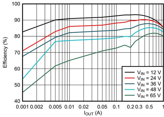
$f_{SW} = 400\text{ kHz}$      $V_{OUT} = 5\text{ V}$     LMR51610X
