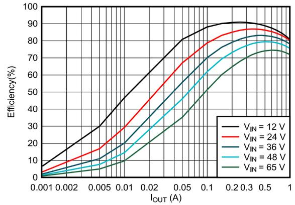
$f_{SW} = 400\text{ kHz}$      $V_{OUT} = 3.3\text{ V}$     LMR51610XF
