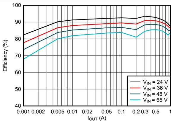
$f_{SW} = 1.1\text{ MHz}$      $V_{OUT} = 12\text{ V}$     LMR51610Y
