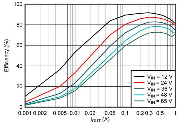
$f_{SW} = 1.1\text{ MHz}$      $V_{OUT} = 5\text{ V}$     LMR51610YF
