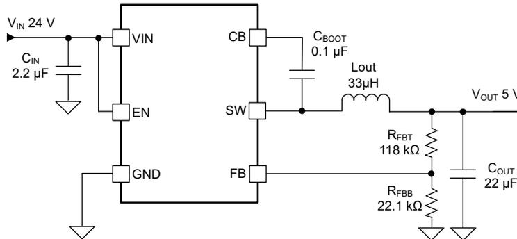
**Figure 8-1. Application Circuit**
