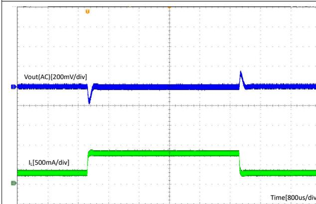
**Figure 8-7. Load Transient (0.25 A – 0.75 A)**
