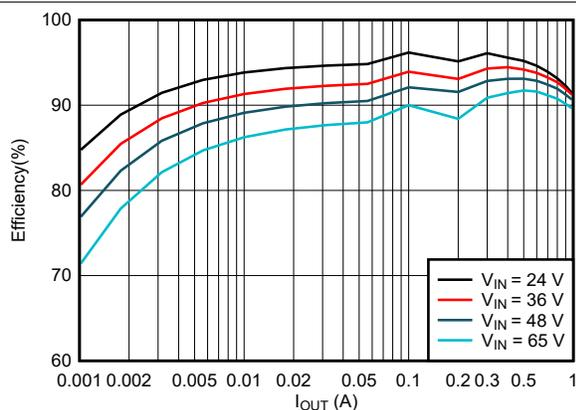
$f_{SW} = 400\text{ kHz}$      $V_{OUT} = 12\text{ V}$     LMR51610X
