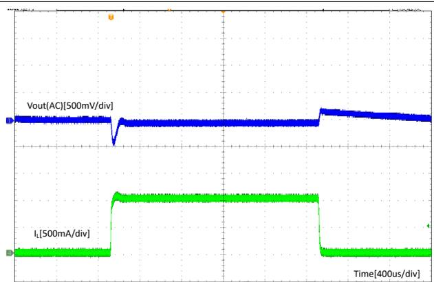
**Figure 8-8. Load Transient (0 A – 1 A)**
