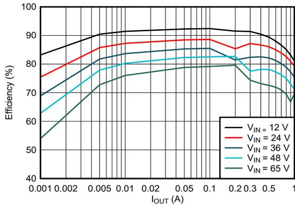
$f_{SW} = 1.1\text{ MHz}$      $V_{OUT} = 5\text{ V}$     LMR51610Y
