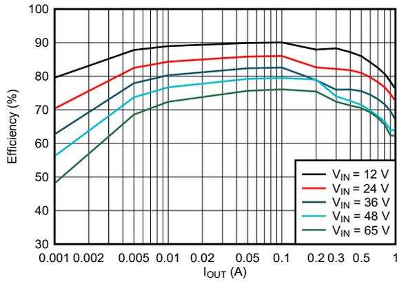
$f_{SW} = 1.1\text{ MHz}$      $V_{OUT} = 3.3\text{ V}$     LMR51610Y
