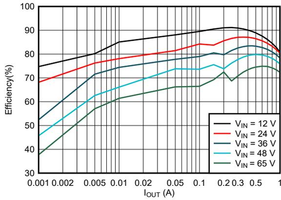
$f_{SW} = 400\text{ kHz}$      $V_{OUT} = 3.3\text{ V}$     LMR51610X
