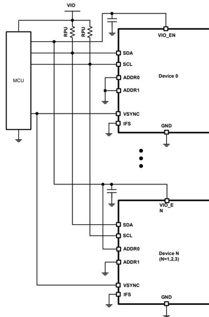
**Figure 7-16. I<sup>2</sup>C Multiple Devices Connection**
