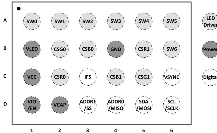
Figure 5-1. LP5867 YBH Package 24-Pin WCSP Top View
