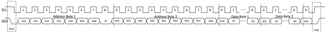
**Figure 7-14. I<sup>2</sup>C Write Timing**
