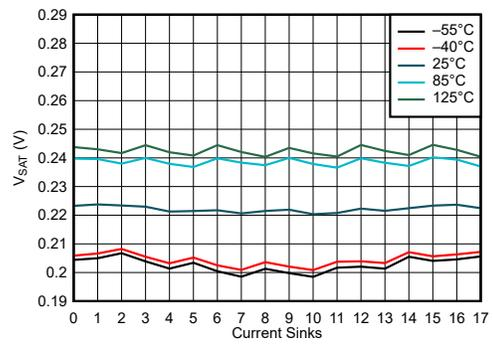
Figure 6-8.  $V_{SAT}$  vs Current Sinks (10mA)
