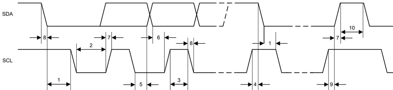
**Figure 6-2. I<sup>2</sup>C Timing Parameters**
