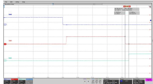
Switch blank time  $t_{SW\_BLK} = 0.5\mu s$
