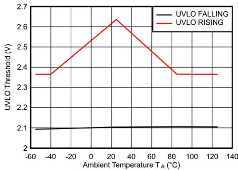
Figure 6-3.  $V_{CC}$  UVLO Rising and Falling Thresholds
