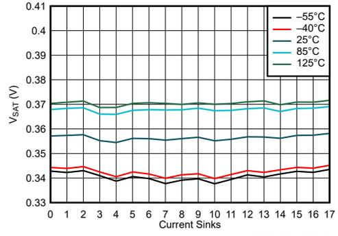
Figure 6-6.  $V_{SAT}$  vs Current Sinks (50mA)
