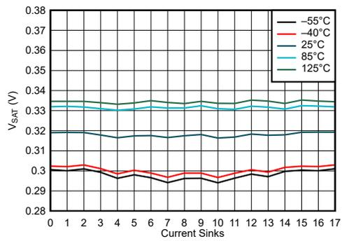
Figure 6-7.  $V_{SAT}$  vs Current Sinks (30mA)
