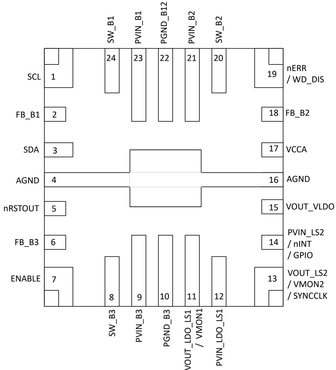
Figure 5-1. Package 24-Pin VQFN-HR Top View
