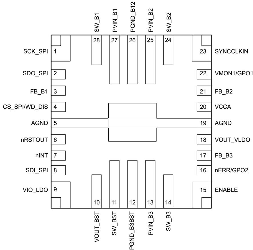
**Figure 5-1. RXV Package, 28-Pin VQFN-HR (Top View)**
