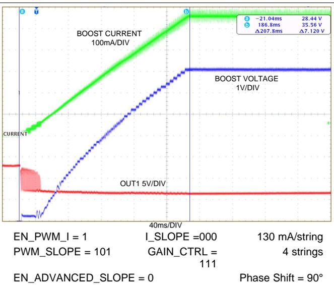
Figure 59. Slope With Hybrid Dimming and Phase Shift
