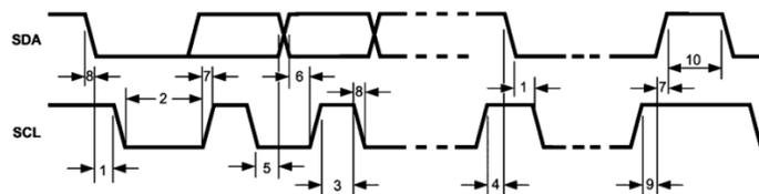
Figure 1. I<sup>2</sup>C Timing
