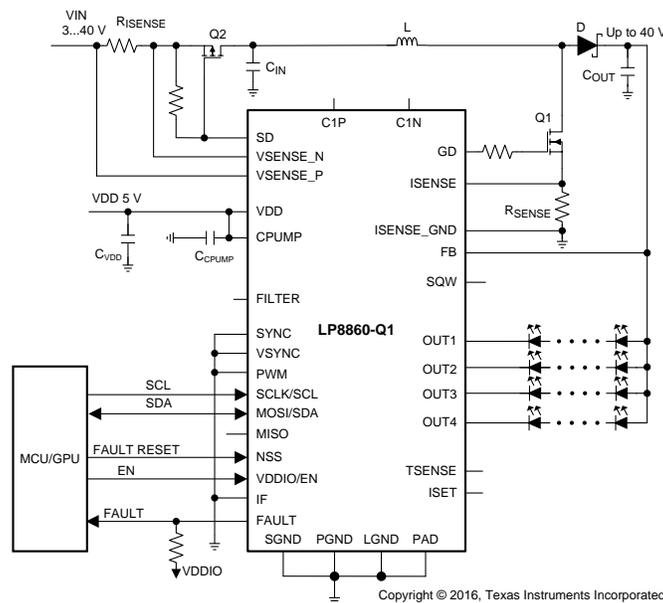
**Figure 53. VDD = 5 V, I<sup>2</sup>C, 4 LED Outputs in Display Mode**
