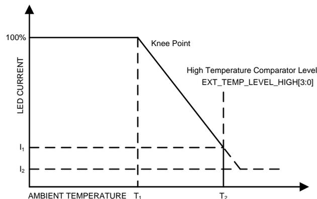
**Figure 33. Current Dimming for High Ambient Temperature**
