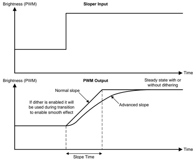
Figure 14. Sloper Operation
