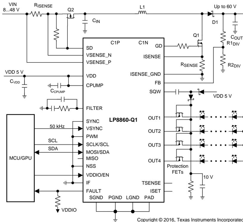
Figure 61. VDD = 5 V, I<sup>2</sup>C, High-Voltage Output with Output Protection FETs Circuits
