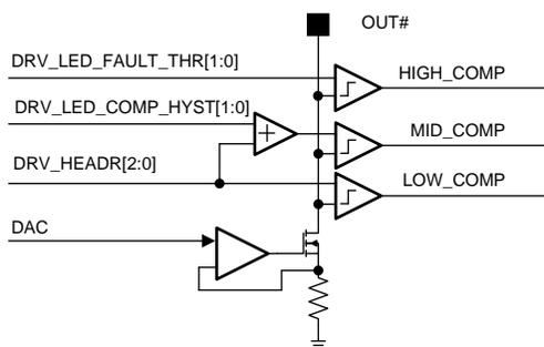
Figure 28. Output Voltage Comparators
