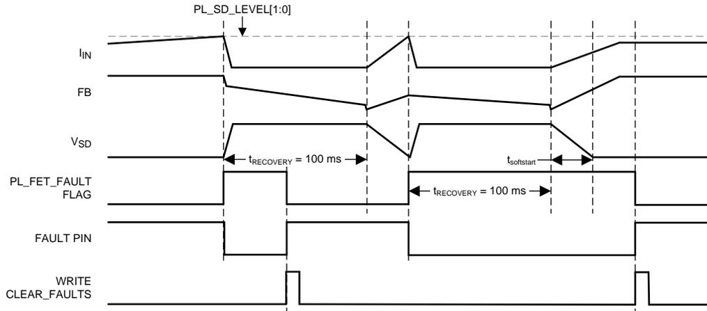
Figure 39. Input OVP Triggering and Recovery
