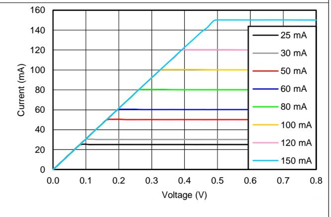
Figure 6. LED Current vs Headroom Voltage
