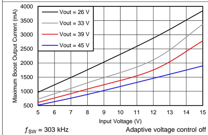
Figure 5. Boost Maximum Output Current
