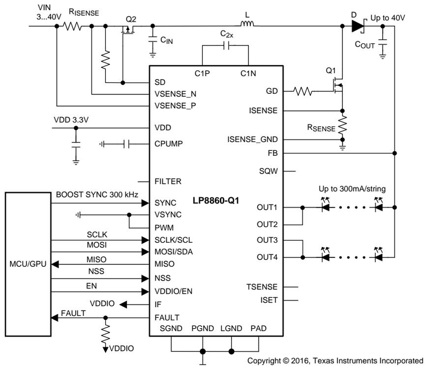
Figure 62. Two Channels at 300 mA/String, VDD = 3.3 V, SPI
