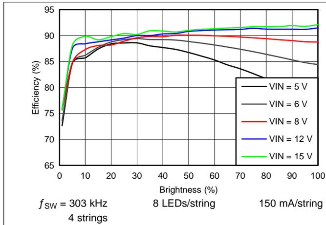
Figure 3. System Efficiency
