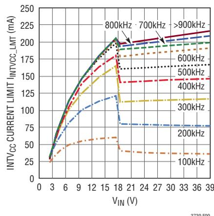
Figure 9. INTV<sub>CC</sub> Current Limit vs V<sub>IN</sub>, f<sub>sw</sub>
