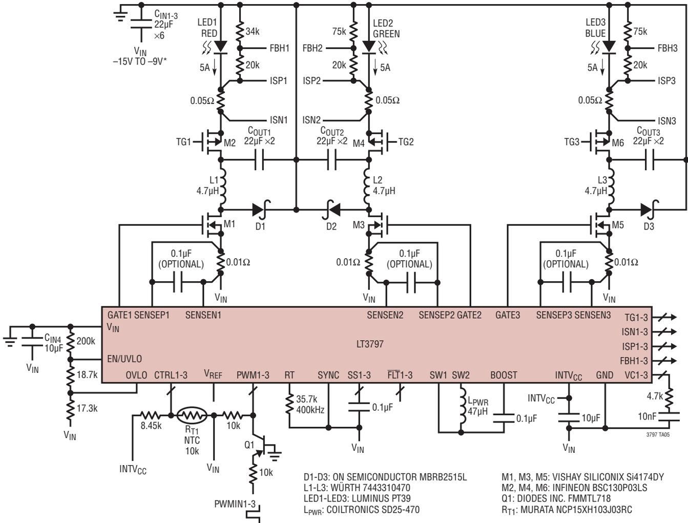
\*NEGATIVE INPUT VOLTAGE IS NECESSARY BECAUSE THE COMMON ANODES OF THE LEDS OF THIS APPLICATION NEED TO BE CONNECTED TO GND
