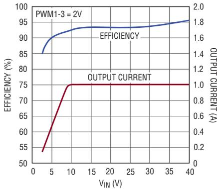
500:1 PWM Dimming at 120Hz
