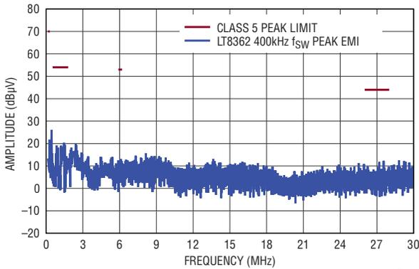
12V INPUT TO 48V OUTPUT AT 300mA,  $f_{SW} = 400\text{kHz}$
