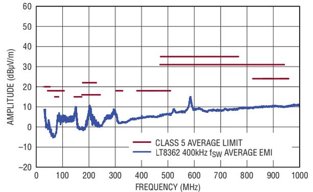
12V INPUT TO 48V OUTPUT AT 300mA,  $f_{SW} = 400\text{kHz}$
