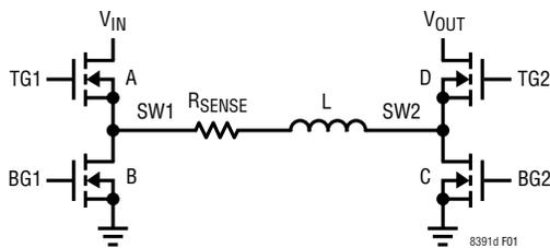
Figure 1. Simplified Diagram of the Power Switches
