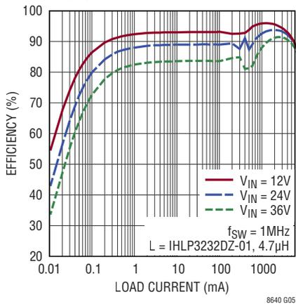
LT8643S Low Load Efficiency at 5V<sub>OUT</sub>
