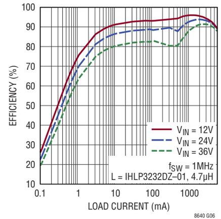
LT8640S Low Load Efficiency at 3.3V<sub>OUT</sub>
