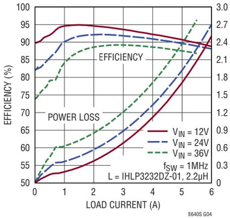
LT8640S Low Load Efficiency at 5V<sub>OUT</sub>
