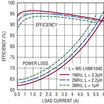
12V<sub>IN</sub> to 3.3V<sub>OUT</sub> Efficiency vs Frequency
