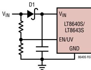
Figure 7. Reverse  $V_{IN}$  Protection
