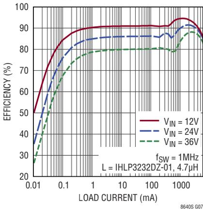
LT8643S Low Load Efficiency at 3.3V<sub>OUT</sub>
