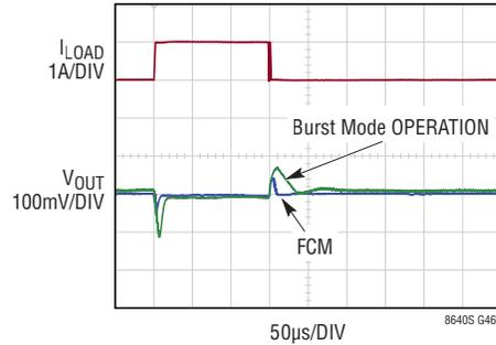
C<sub>C</sub> = 330pF, R<sub>C</sub> = 6.49k, C<sub>LEAD</sub> = 4.7pF
