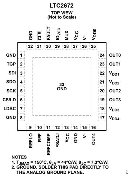
Figure 5. LFCSP Pin Configuration
