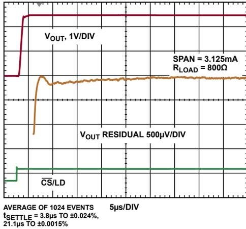
Figure 13. Settling 0 mA to 3.125 mA Step
