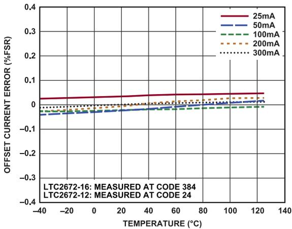
Figure 15. Offset Current Error vs. Temperature
