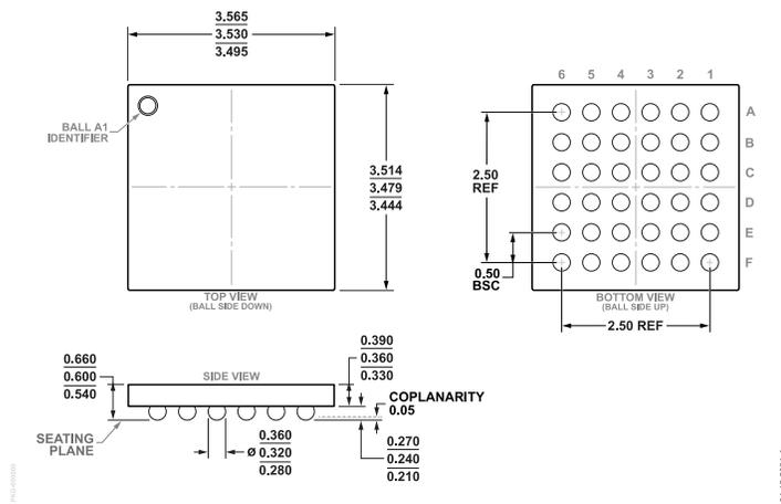
Figure 37. 36-Ball Wafer Level Chip Scale Package [WLCSP]
