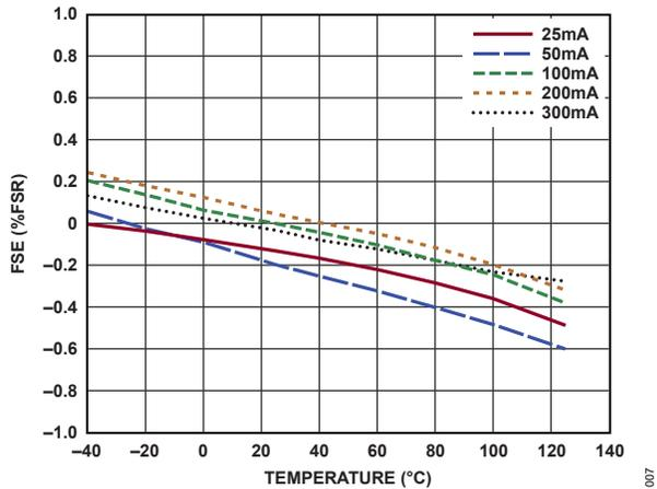
Figure 9. Full-Scale Current Error (FSE) vs Temperature
