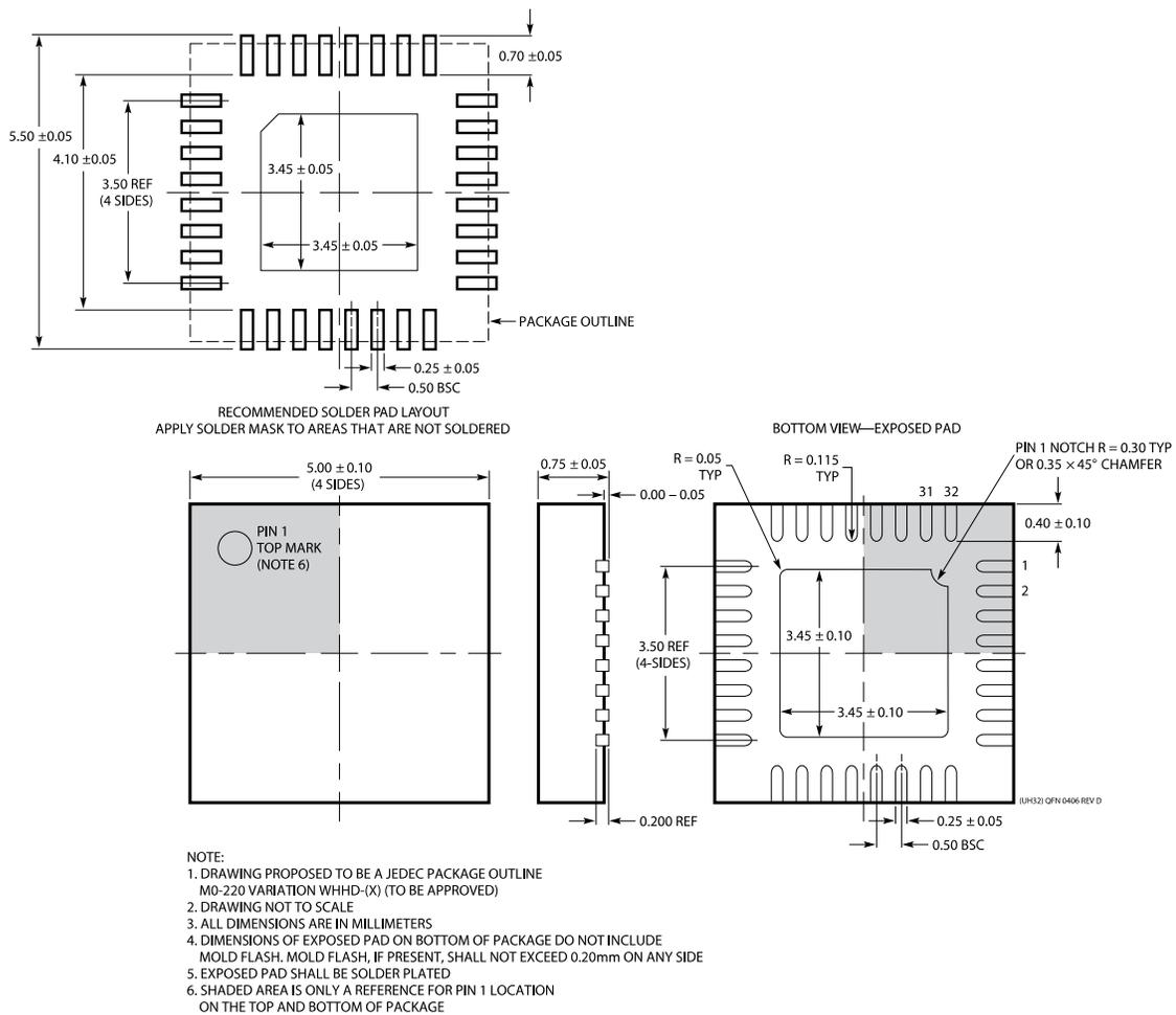
Figure 36. 32-Lead Plastic QFN
