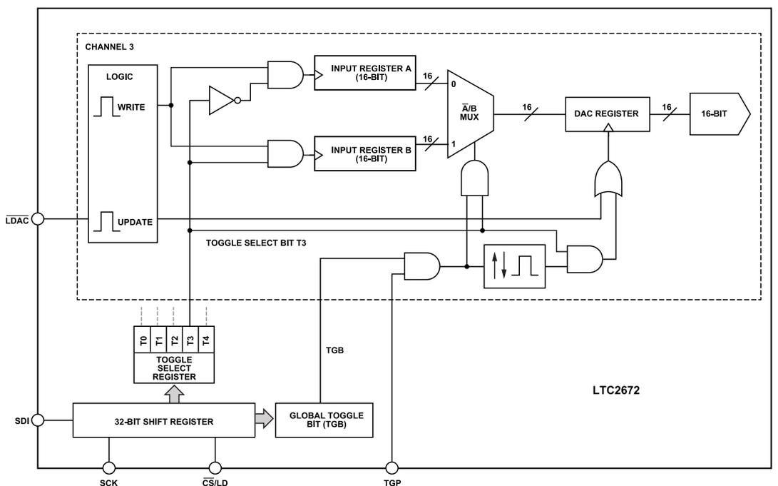
Figure 31. Conceptual Block Diagram, Toggle Functionality
