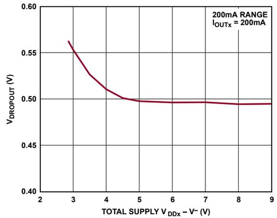
Figure 17.  $V_{DROP-OUT}$  vs. Total Supply  $V_{DDx} - V^-$
