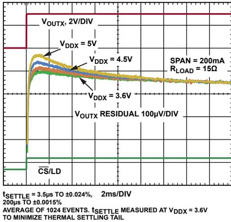
Figure 14. Settling 0 mA to 200 mA Step
