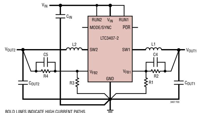
Figure 3. LTC3407-2 Layout Diagram (See Board Layout Checklist)
