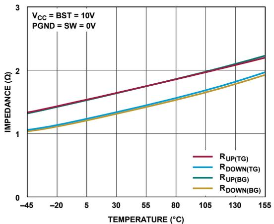
Figure 14. TG/BG Pull-Up and Pull-Down Resistance vs. Temperature
