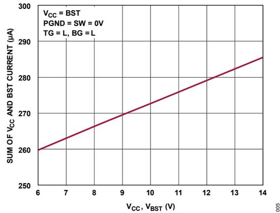
Figure 5. Total Supply Current vs. Supply Voltage
