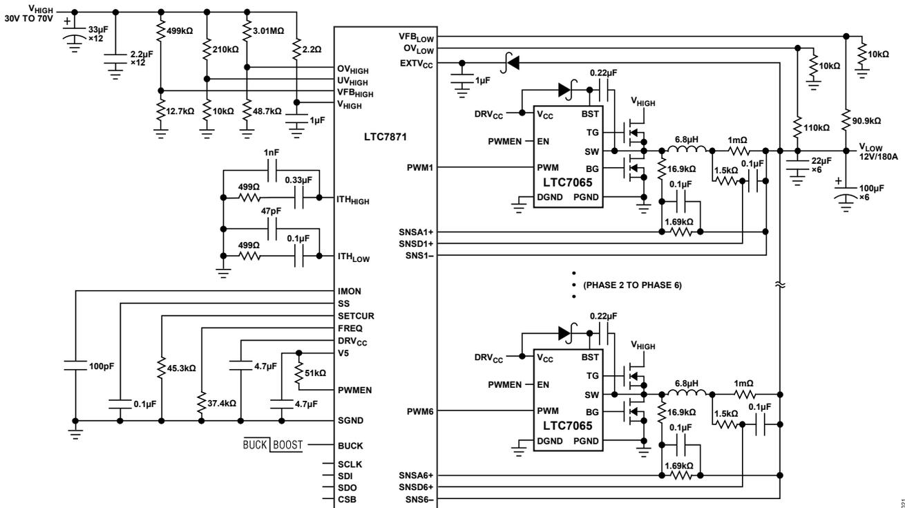
Figure 18. 6-Phase 12V/180A Converter with the LTC7065 and MOSFETs Using LTC7871
