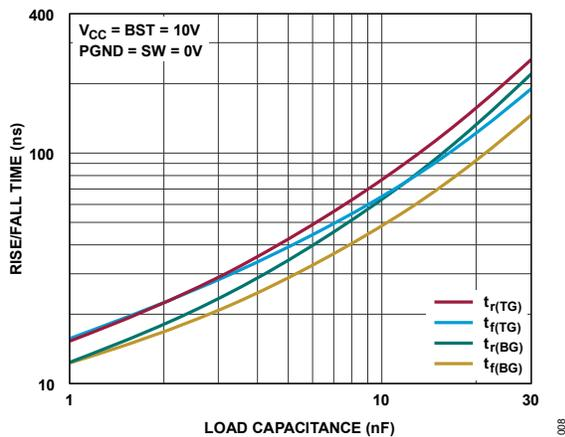
Figure 8. Rise and Fall Time vs. Load Capacitance
