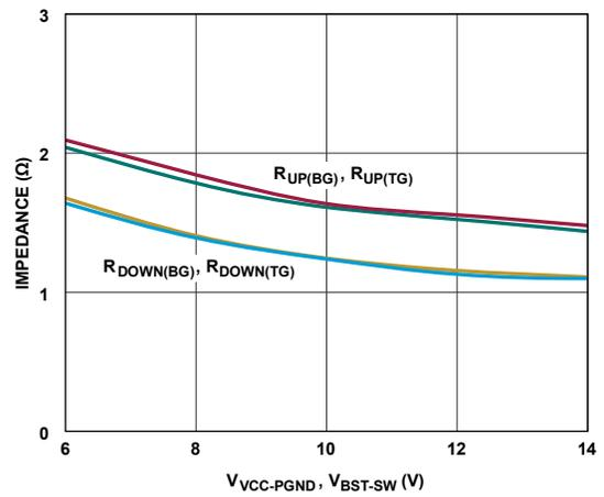
Figure 13. TG/BG Pull-Up and Pull-Down Resistance vs. Driver Supply Voltage
