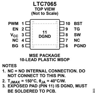
Figure 3. Pin Configurations and Function Descriptions
