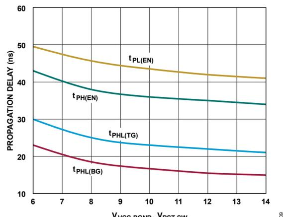
Figure 9. Propagation Delay vs. Driver Supply Voltage
