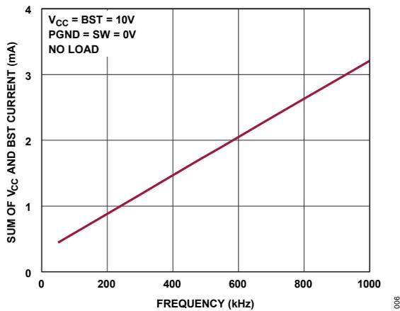
Figure 6. Total Supply Current vs. Input Frequency
