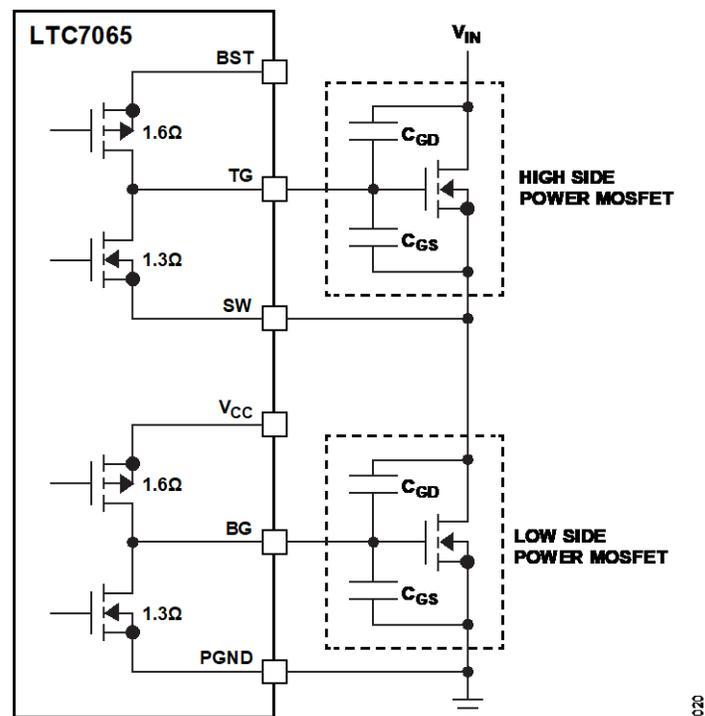
Figure 17. Simplified Output Stage in Half-Bridge Configuration
