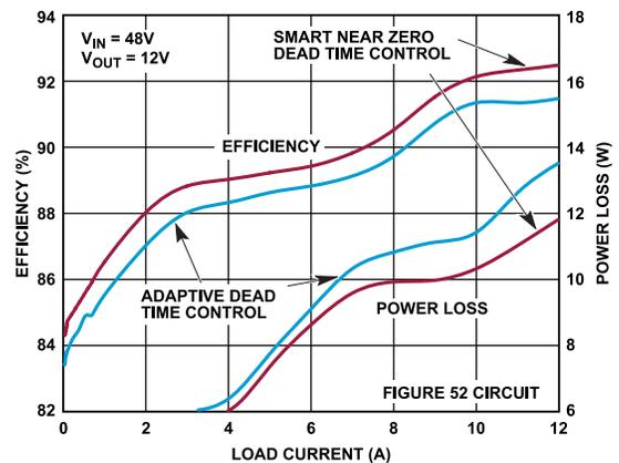
Figure 2. Efficiency and Power Loss vs. Load Current
