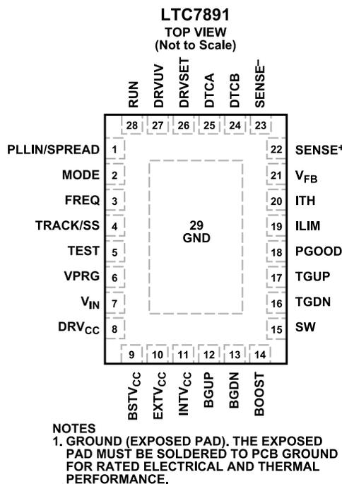
Figure 3. Pin Configuration
