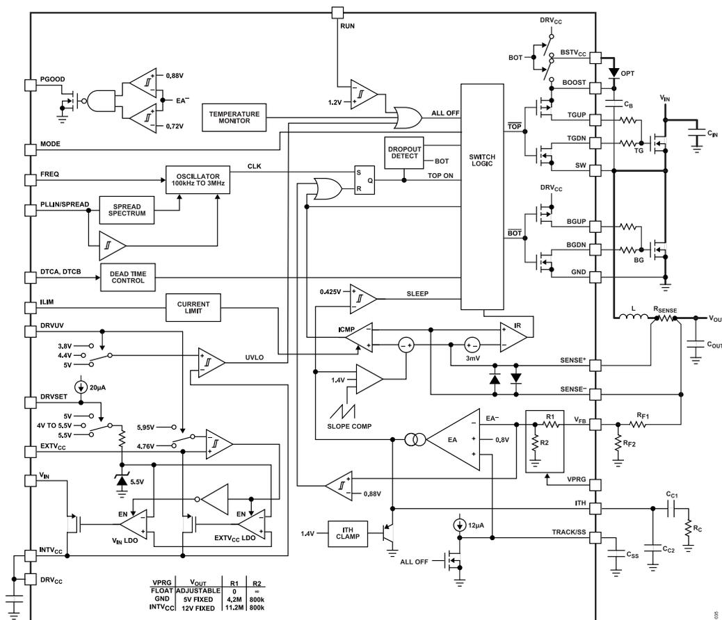
Figure 35. Functional Diagram
