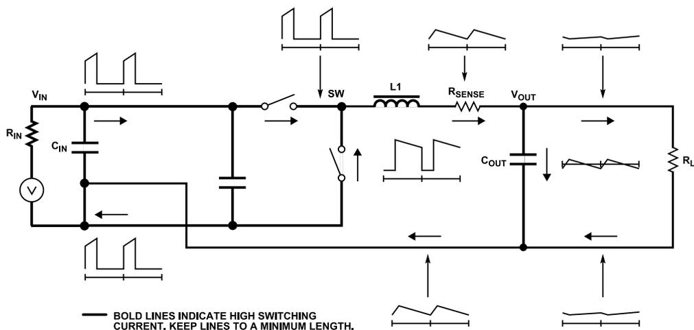
Figure 51. Branch Current Waveform
