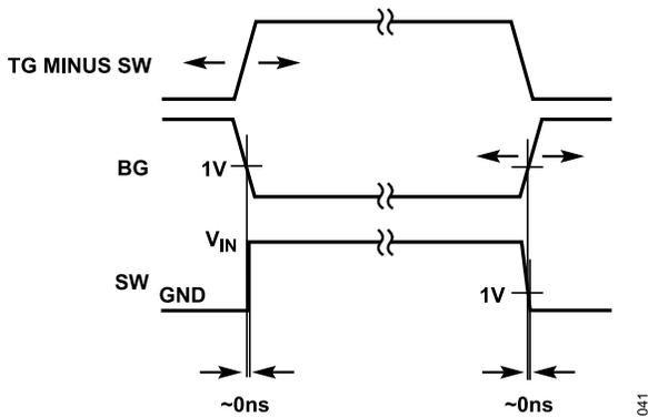
Figure 41. DTCx Pins Tied to INTV<sub>CC</sub>—Smart Near Zero Dead Time Control
