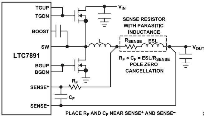
Figure 37. Using a Resistor to Sense Current
