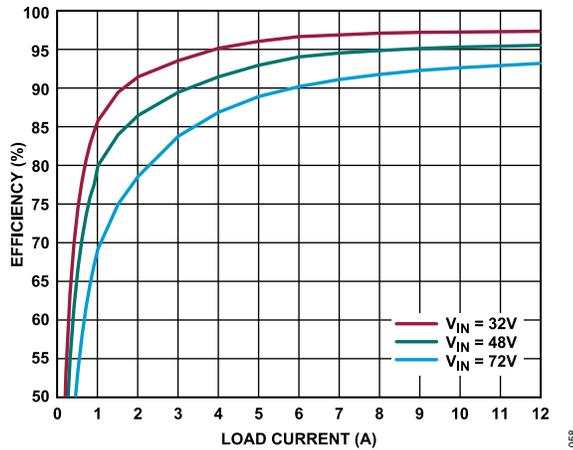
Figure 57. V<sub>OUT</sub> Efficiency vs. Load Current for Figure 56
