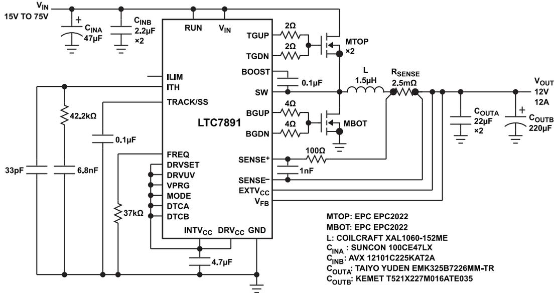
Figure 52. High Efficiency, 12 V<sub>OUT</sub>, 12 A, 1 MHz, Step-Down Regulator Using GaN FETs
