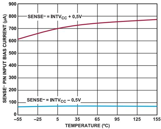
Figure 14.  $SENSE^-$  Pin Input Bias Current vs. Temperature
