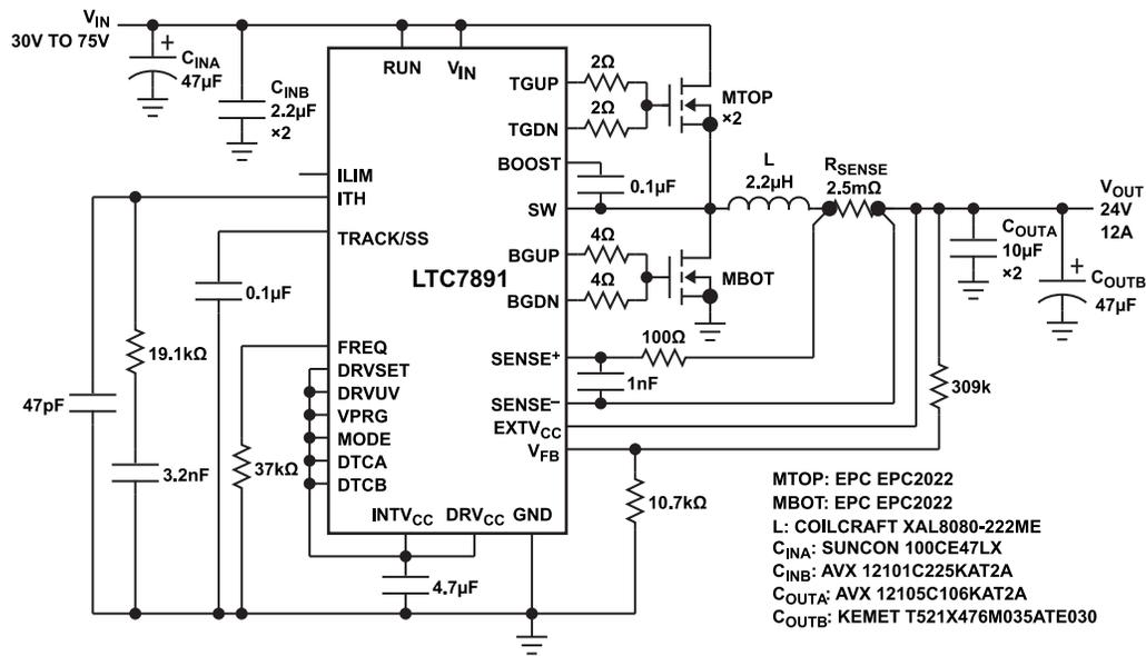
Figure 56. High Efficiency, 24 V<sub>OUT</sub>, 1 MHz, Step-Down Regulator Using GaN FETs
