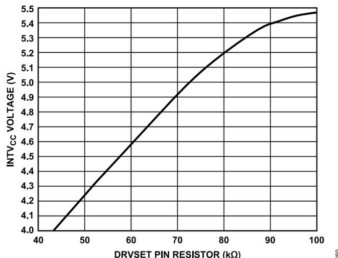
Figure 50. Relationship Between INTV<sub>CC</sub> Voltage and Resistor Value at the DRVSET Pin
