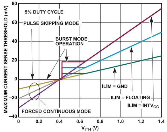
Figure 13. Maximum Current Sense Threshold vs.  $V_{ITH}$
