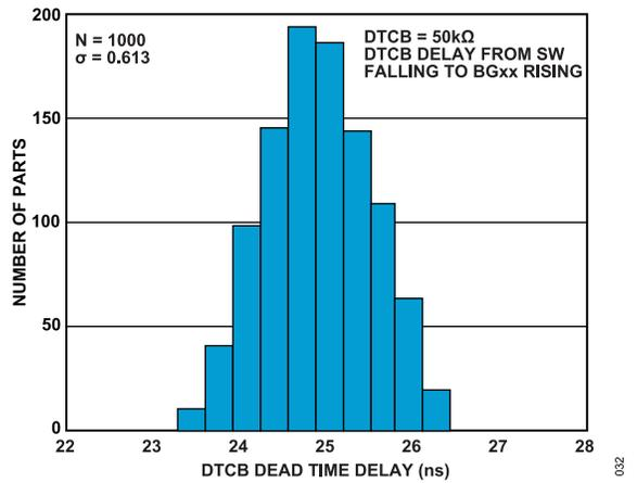
Figure 32. DTCB = 50 kΩ Dead Time Delay Histogram
