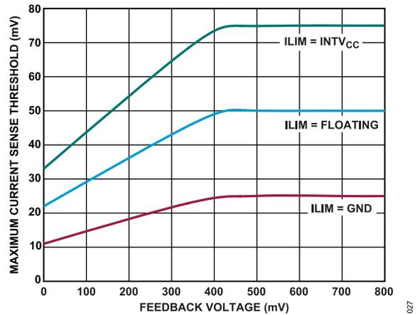
Figure 27. Maximum Current Sense Threshold vs. Feedback Voltage
