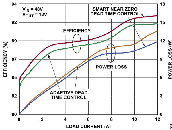
Figure 53. V<sub>OUT</sub> Efficiency and Power Loss vs. Load Current for Figure 52
