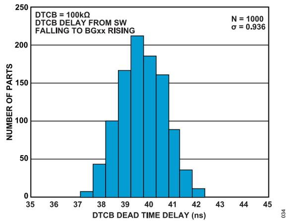
Figure 34. DTCB = 100 kΩ Dead Time Delay Histogram
