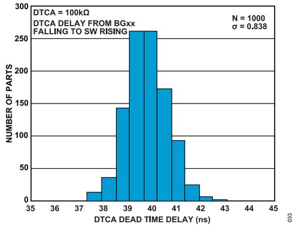
Figure 33. DTCA = 100 kΩ Dead Time Delay Histogram
