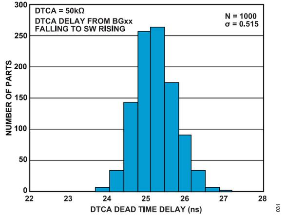
Figure 31. DTCA = 50 kΩ Dead Time Delay Histogram
