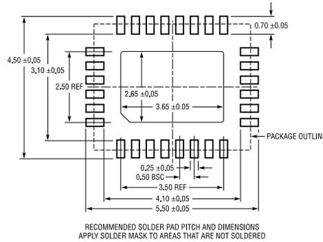
Figure 59. 28-Lead Plastic Side Wettable QFN
