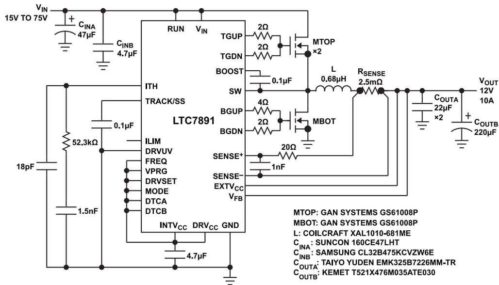
Figure 54. High Efficiency 12 V<sub>OUT</sub>, 10 A, 2 MHz, Step-Down Regulator Using GaN FETs
