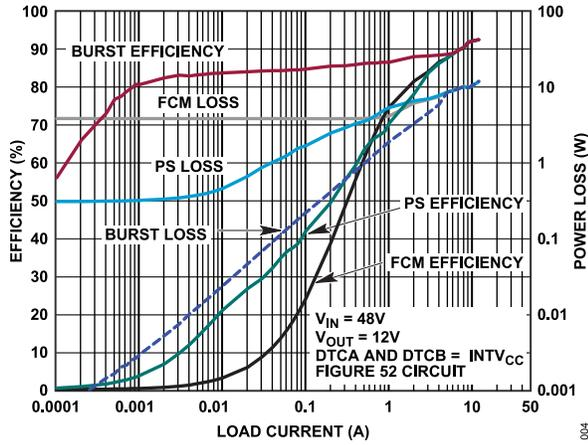
Figure 4. Efficiency and Power Loss vs. Load Current
