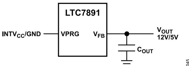
Figure 45. Setting Fixed 12 V or 5 V Voltage
