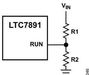
Figure 46. Using the RUN Pin as a UVLO
