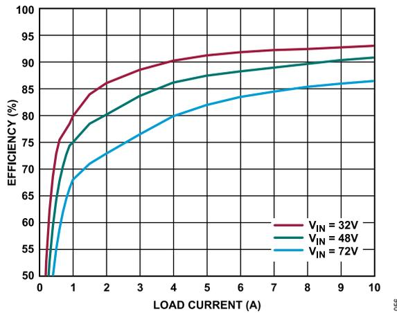
Figure 55. V<sub>OUT</sub> Efficiency vs. Load Current for Figure 54
