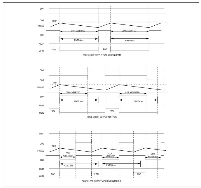
Figure 2. CDR Monitor Timing Diagram
