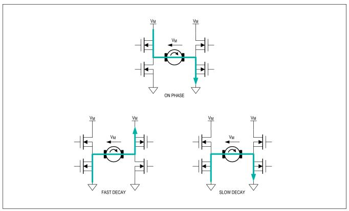
Figure 3. Current Flow During ON and Decay Modes
