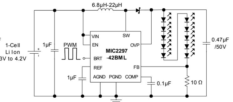
10 Series LED Driver with PWM Brightness Control
