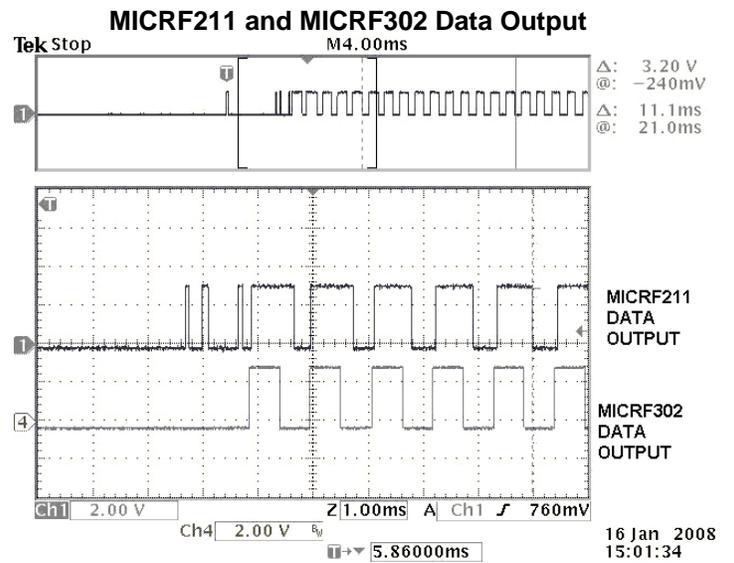
Figure 10. Micrel Receiver Example Receiving MICRF302 Data Output
