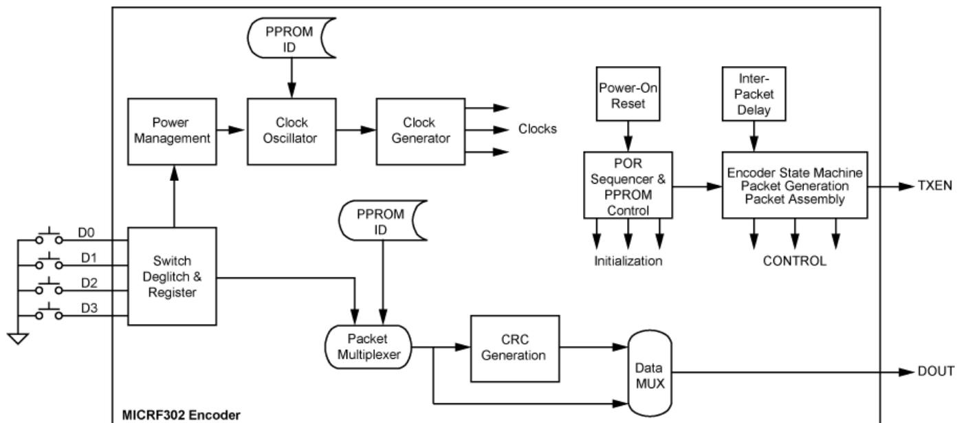
Figure 3. MICRF302 Parallel Encoder Functional Diagram
