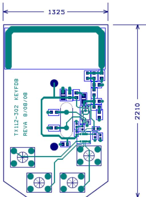
Figure 15. TX112-MICRF302 KEYFOB Evaluation Board, Top View
