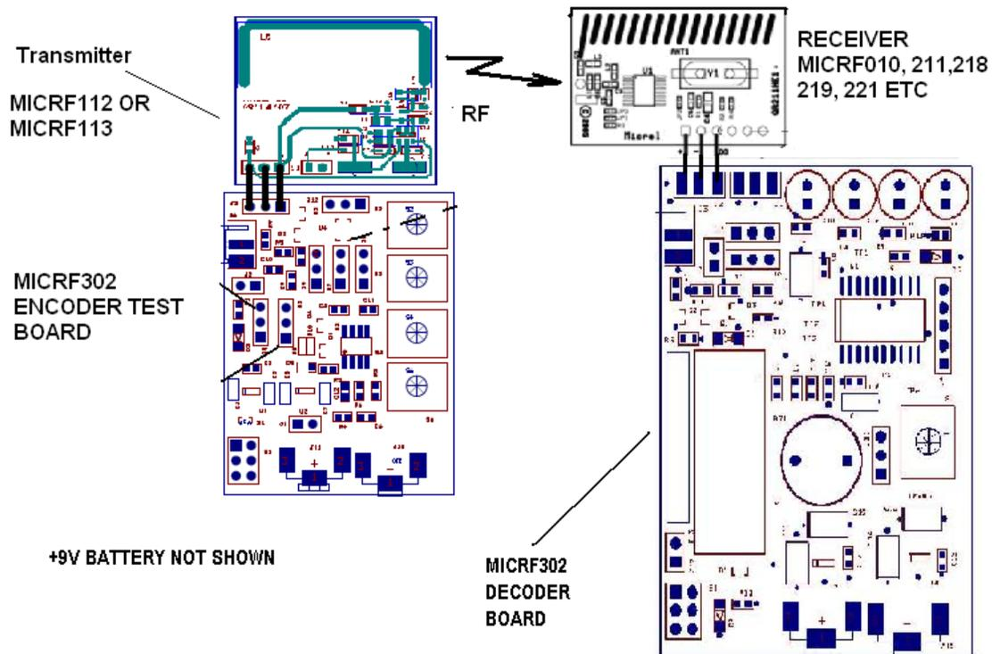
Figure 13. Test Configuration
