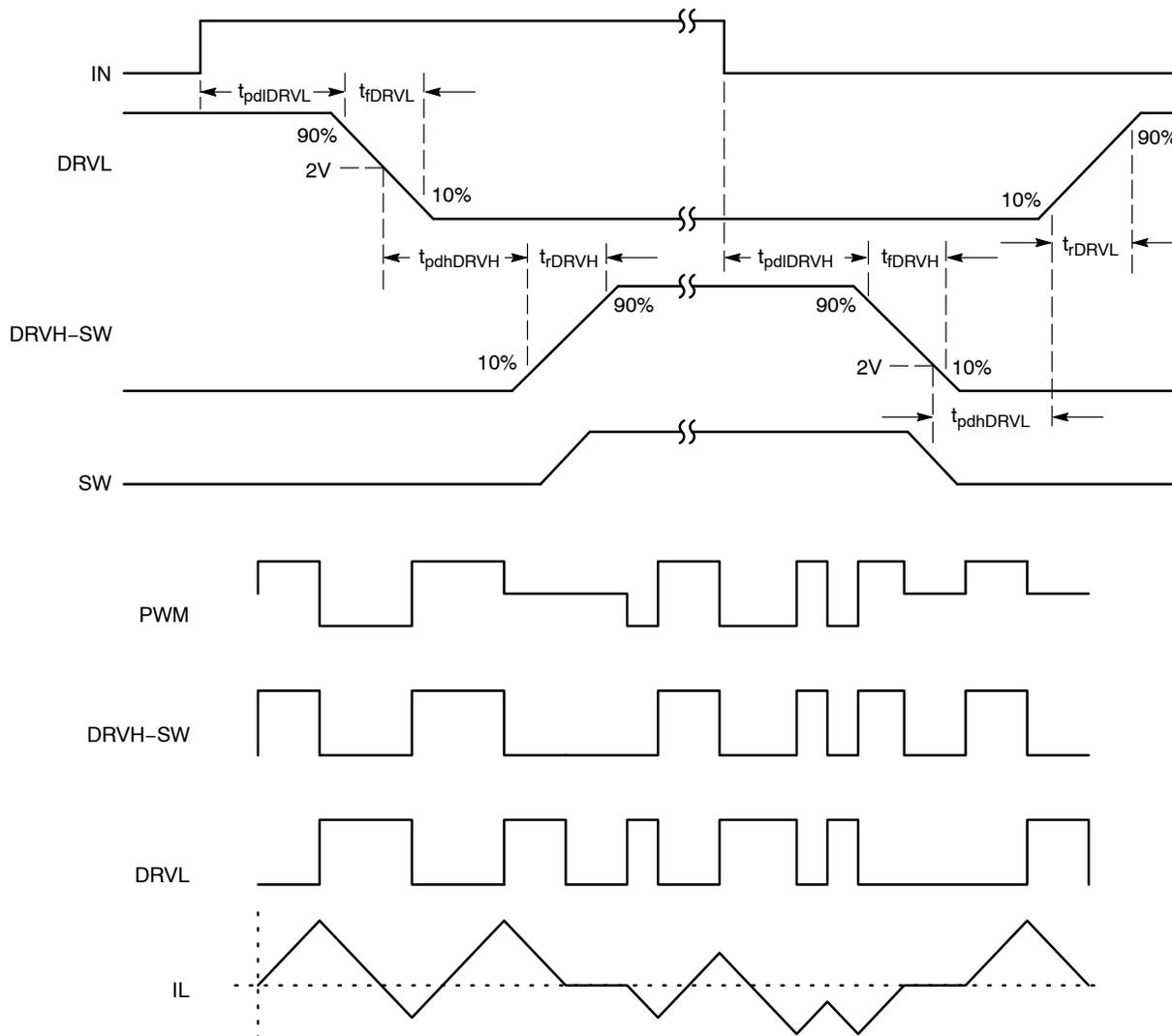
**Figure 3. Timing Diagram**
