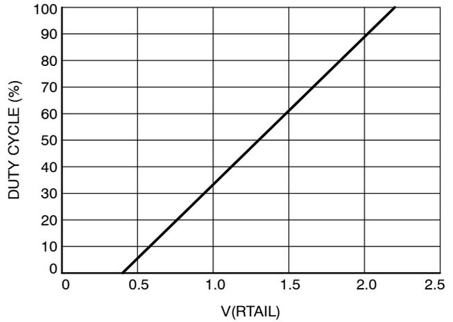
Figure 14. Duty Cycle vs. V(R<sub>TAIL</sub>)
