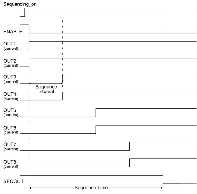
**Figure 8. Sequencing Timing Diagram (SEQ1 = 1, SEQ2 = 0)**
