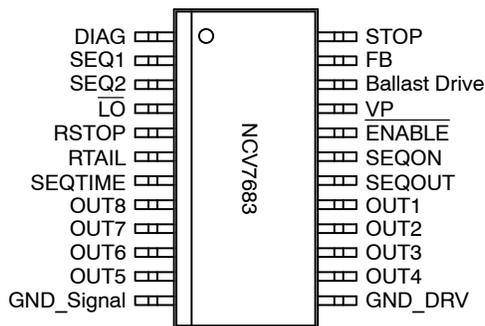
Figure 2. Pinout Diagram
