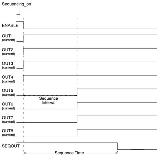
**Figure 9. Sequencing Timing Diagram (SEQ1 = 0, SEQ2 = 1)**
