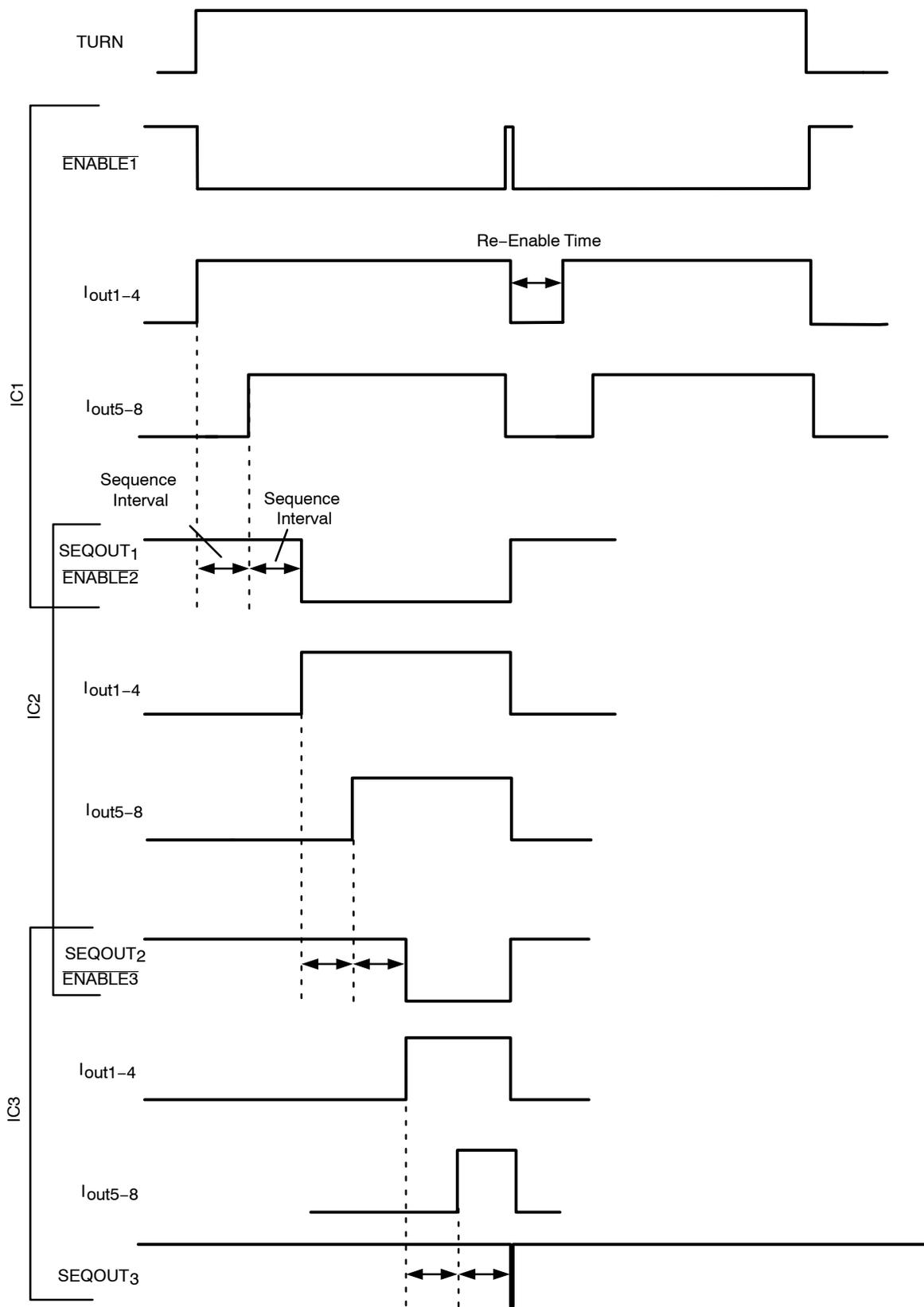
Figure 36. Sequencing Timing Diagram with Re-Enable Time Delay
