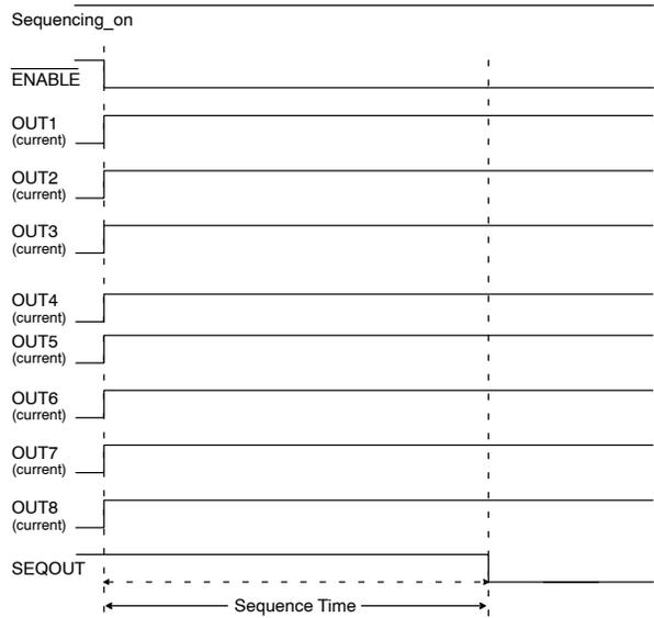
**Figure 10. Sequencing Timing Diagram (SEQ1 = 1, SEQ2 = 1)**
