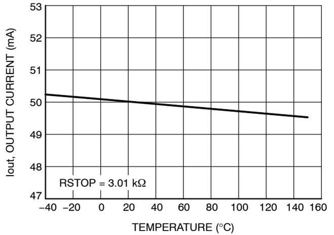
Figure 12. I<sub>out</sub> vs. Temperature
