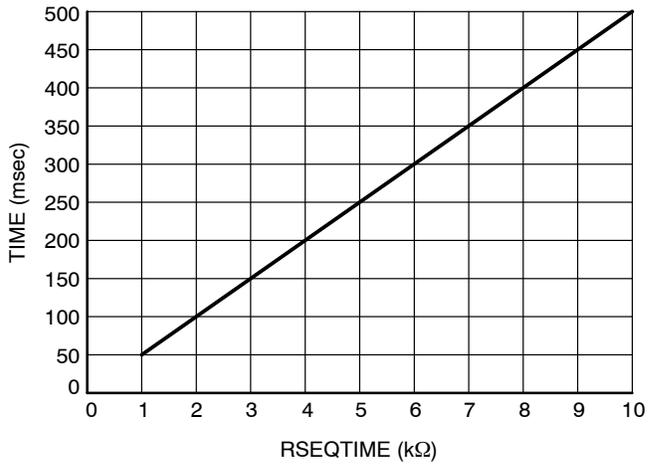
Figure 21. (Sequence Time / Re-Enable Time) vs.  $R_{SEQTIME}$
