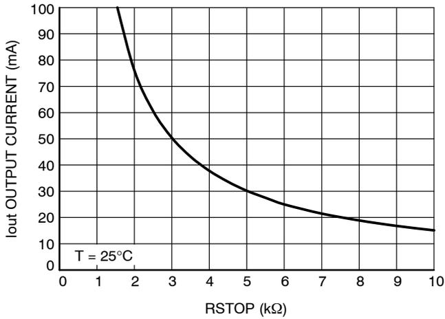
Figure 11. I<sub>out</sub> vs. R<sub>STOP</sub>
