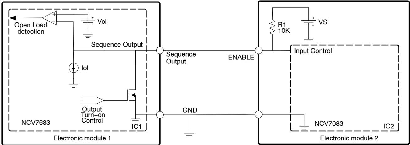
Figure 31. Daisy Chain Interface between Multiple ICs
