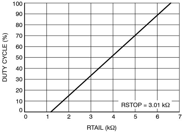
Figure 13. Duty Cycle vs. R<sub>TAIL</sub>
