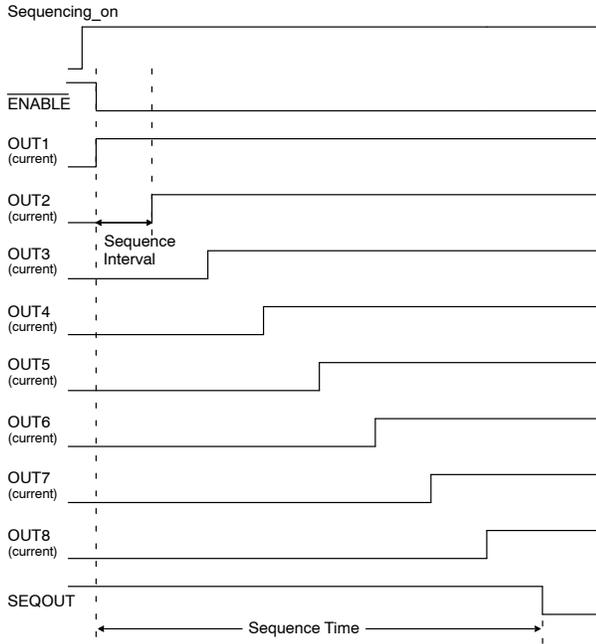
**Figure 7. Sequencing Timing Diagram (SEQ1 = 0, SEQ2 = 0)**
