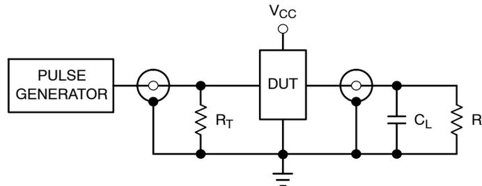
$$R_T = Z_{OUT} \text{ of pulse generator (typically } 50 \Omega)$$
