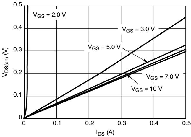
Figure 2.  $V_{DS(on)}$  Variation with  $I_{DS}$  and Gate Voltage
