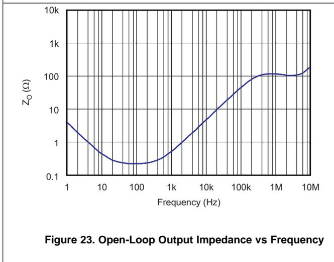
Figure 23. Open-Loop Output Impedance vs Frequency
