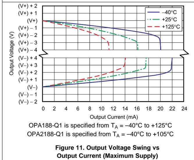
Figure 11. Output Voltage Swing vs Output Current (Maximum Supply)
