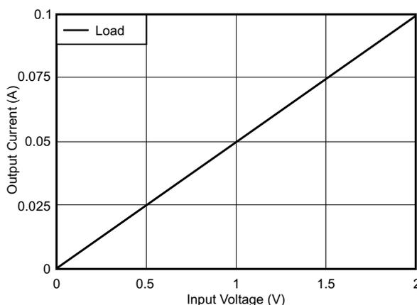
**Figure 44. Measured Transfer Function for High-Side V-I Converter**
