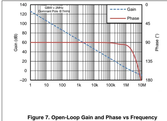
Figure 7. Open-Loop Gain and Phase vs Frequency
