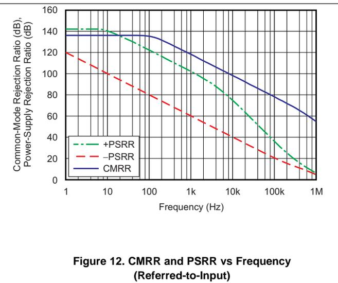
Figure 12. CMRR and PSRR vs Frequency (Referred-to-Input)
