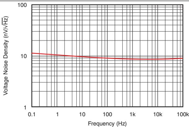
Figure 17. Input Voltage Noise Spectral Density vs Frequency
