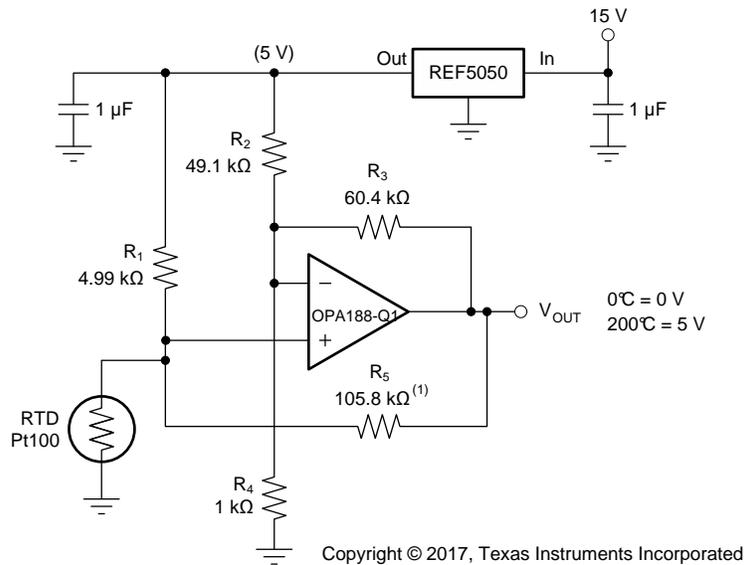
(1)  $R_5$  provides positive-varying excitation to linearize output.
