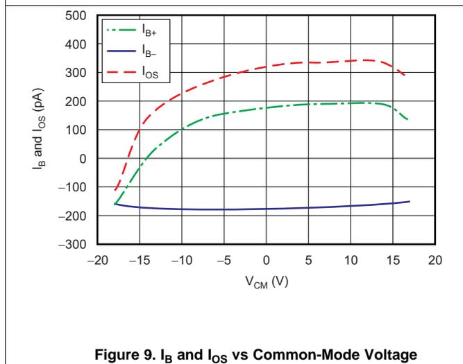
Figure 9.  $I_B$  and  $I_{OS}$  vs Common-Mode Voltage
