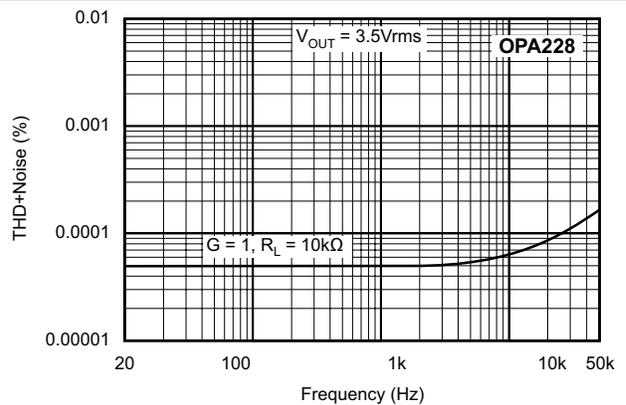
**Figure 6-6. Total Harmonic Distortion + Noise vs Frequency**
