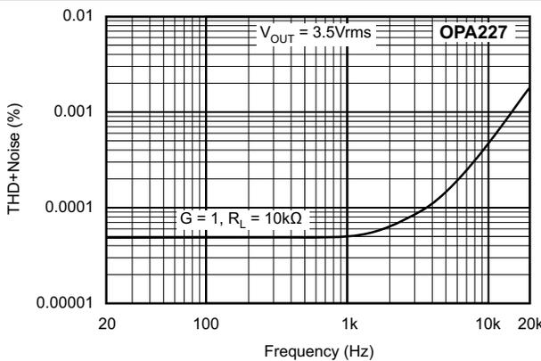
**Figure 6-5. Total Harmonic Distortion + Noise vs Frequency**
