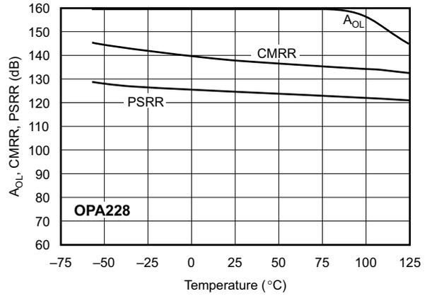
Figure 6-14.  $A_{OL}$ , CMRR, PSRR vs Temperature
