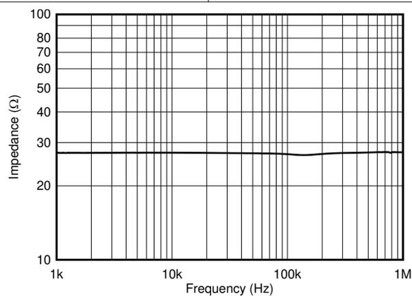
Figure 6-35. Open-loop Output Impedance
