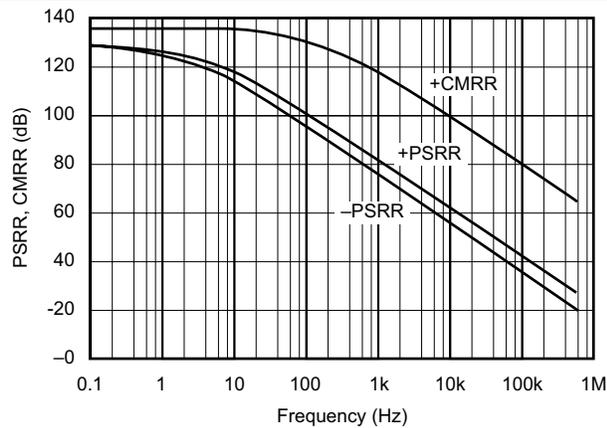
**Figure 6-3. Power Supply and Common-Mode Rejection Ratio vs Frequency**
