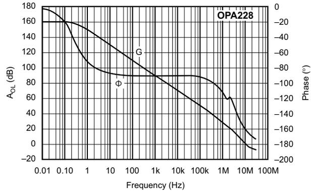
**Figure 6-2. Open-Loop Gain and Phase vs Frequency**
