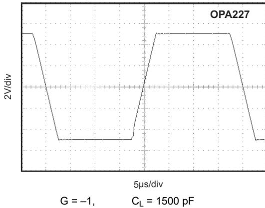
Figure 6-27. Large-Signal Step Response
