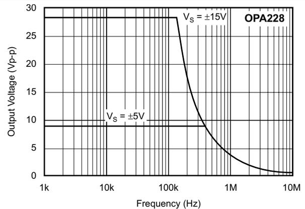
Figure 6-30. Maximum Output Voltage vs Frequency
