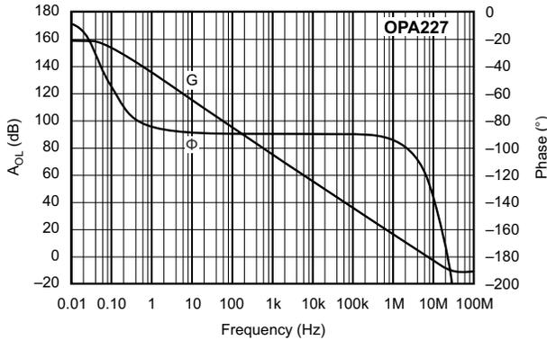
**Figure 6-1. Open-Loop Gain and Phase vs Frequency**
