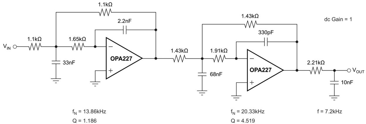
Figure 8-8. Three-Pole, 20 kHz Low Pass, 0.5-dB Chebyshev Filter
