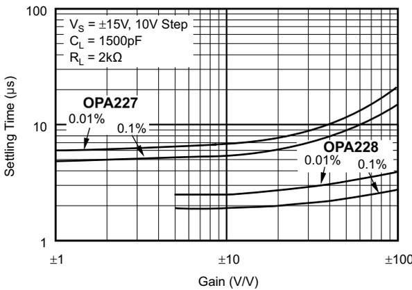
Figure 6-23. Settling Time vs Closed-Loop Gain
