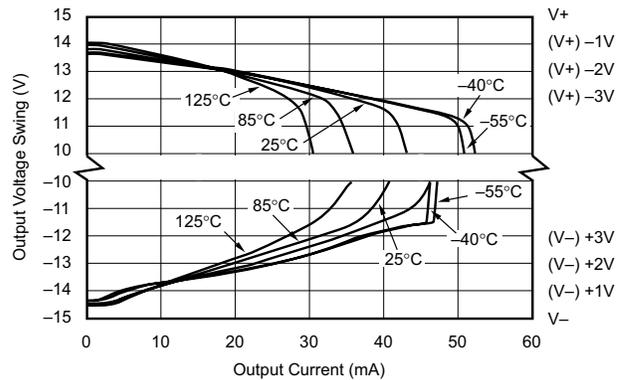
Figure 6-24. Output Voltage Swing vs Output Current
