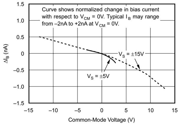
Figure 6-22. Change in Input Bias Current vs Common-Mode Voltage
