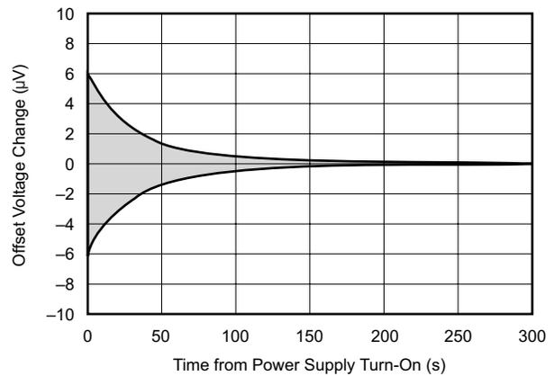
**Figure 6-12. Warm-Up Offset Voltage Drift**
