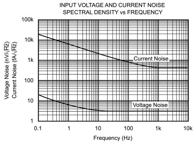
**Figure 6-4. Input Voltage and Current Noise Spectral Density vs Frequency**
