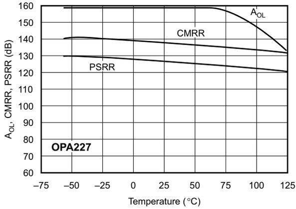
Figure 6-13.  $A_{OL}$ , CMRR, PSRR vs Temperature
