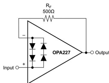
**Figure 7-2. Pulsed Operation**
