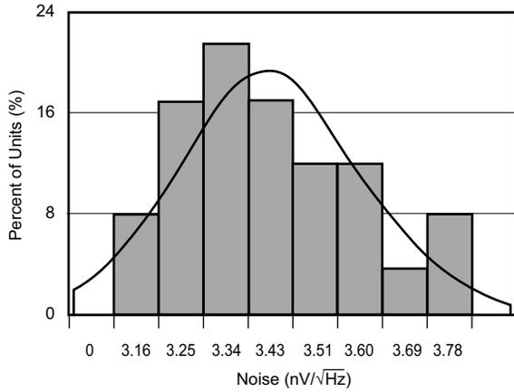
**Figure 6-9. Voltage Noise Distribution (10 Hz)**
