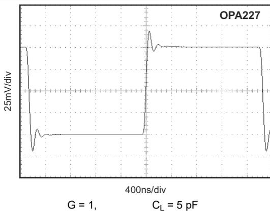
Figure 6-29. Small-Signal Step Response
