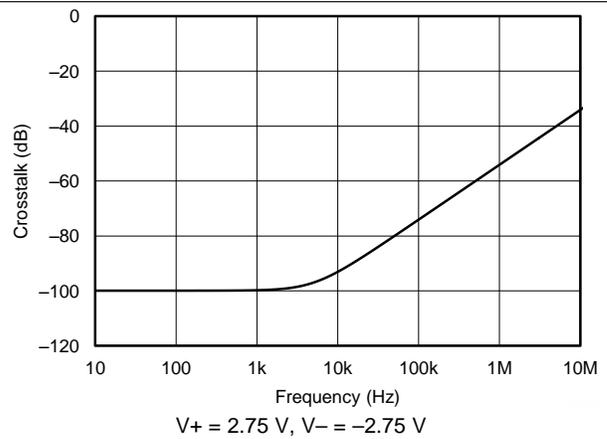
Figure 36. Channel Separation vs Frequency
