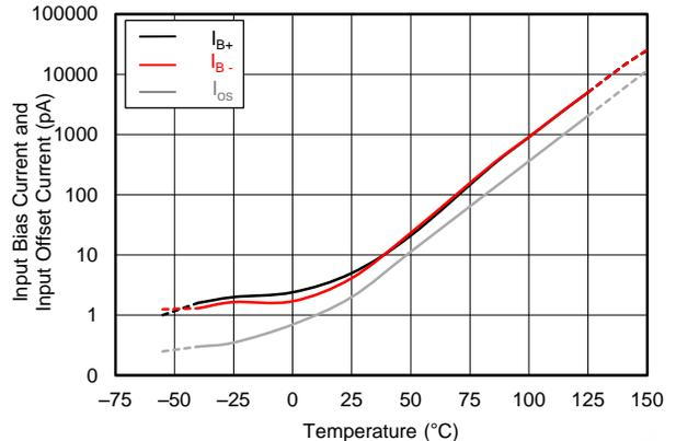
Figure 10. Input Bias and Offset Current vs Temperature
