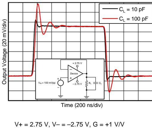
Figure 29. Small-Signal Step Response
