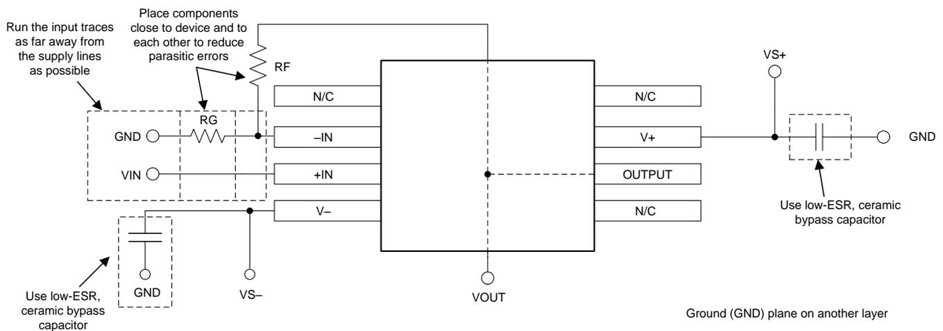
Figure 45. Operational Amplifier Board Layout for Noninverting Configuration
