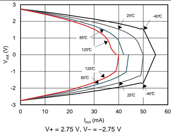
Figure 11. Output Voltage Swing vs Output Current
