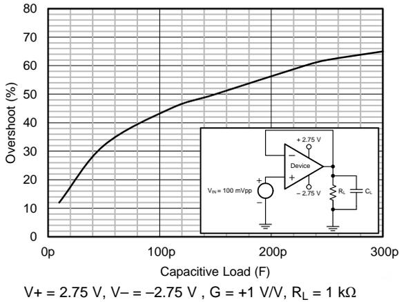
Figure 25. Small-Signal Overshoot vs Load Capacitance
