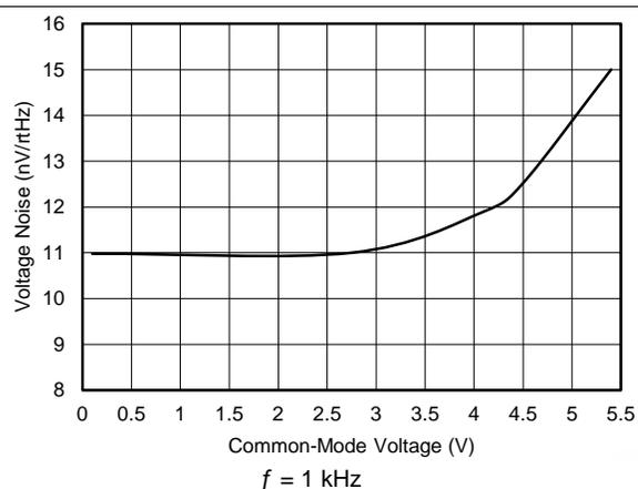
Figure 18. Input Voltage Noise vs Common-Mode Voltage
