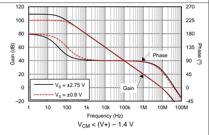
Figure 6. Open-Loop Gain and Phase vs Frequency
