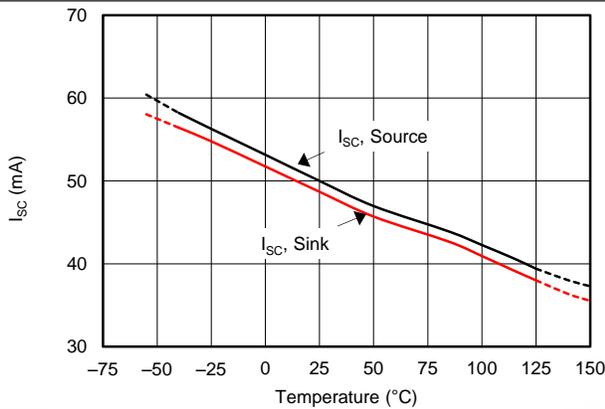
Figure 33. Short-Circuit Current vs Temperature
